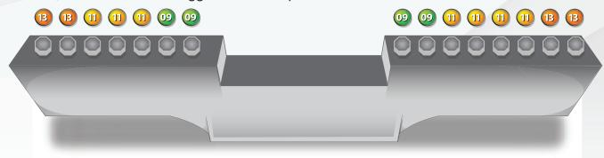
8" & 10", 16 Nozzle - Medium Aggressive set-up 8.08 GPM @ 36K PSI / 8.56 GPM @ 40K PSI
