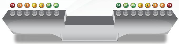
8", & 10", 16 Nozzle - Most Aggressive set-up 8.54 GPM @ 36K PSI / 9.04 GPM @ 40K PSI
