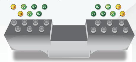
6", 14 Nozzle Spray Bar - 4" lines - Most Aggressive 5.72 GPM @ 36K PSI / 6.06 GPM @ 40K PSI
