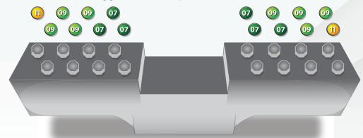
8" & 10", 16 Nozzle - Medium Aggressive set-up 5.4 GPM @ 36K PSI / 5.72 GPM @ 40K PSI
