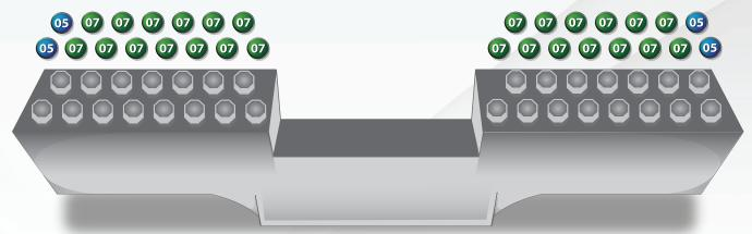
8" & 10", 16 Nozzle Curing Compound Removal set-up - 25,000 - 35,000 PSI
