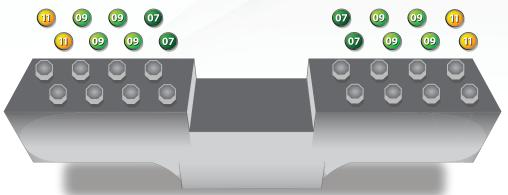
8", & 10", 16 Nozzle - Most Aggressive set-up 5.86 GPM @ 36K PSI / 6.2 GPM @ 40K PSI
