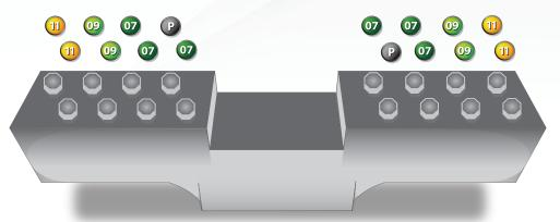
8" & 10", 16 Nozzle - Most Aggressive Set Up 4.88 GPM @ 36K PSI / 5.16 GPM @ 40K PSI
