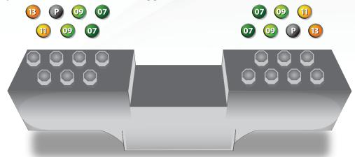
6", 14 Nozzle Spray Bar - 4" Lines - Most Aggressive 4.54 GPM @ 36K PSI / 4.8 GPM @ 40K PSI
