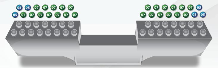
8" & 10", 16 Nozzle - Curing Compound Removal Set-Up - Set Up - 25K - 35K PSI
