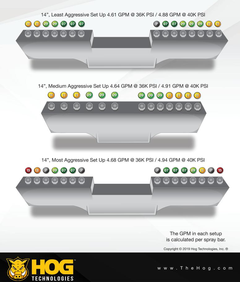
(These configurations are to be used as a general guide for flat line marking removal which may need to be altered to suit your situation.)
