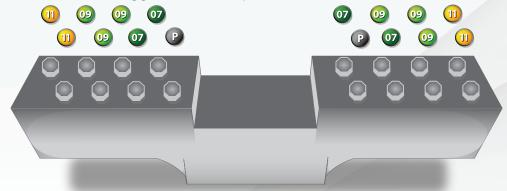
8" & 10", 16 Nozzle - Medium Aggressive Set Up 4.48 GPM @ 36K PSI / 4.74 GPM @ 40K PSI
