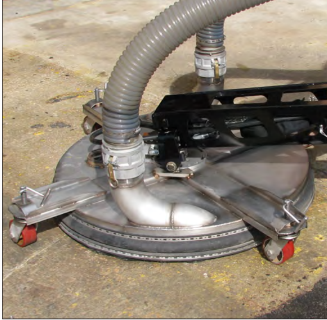
Hog Head Shroud, Caster Wheels & Wear Brush
