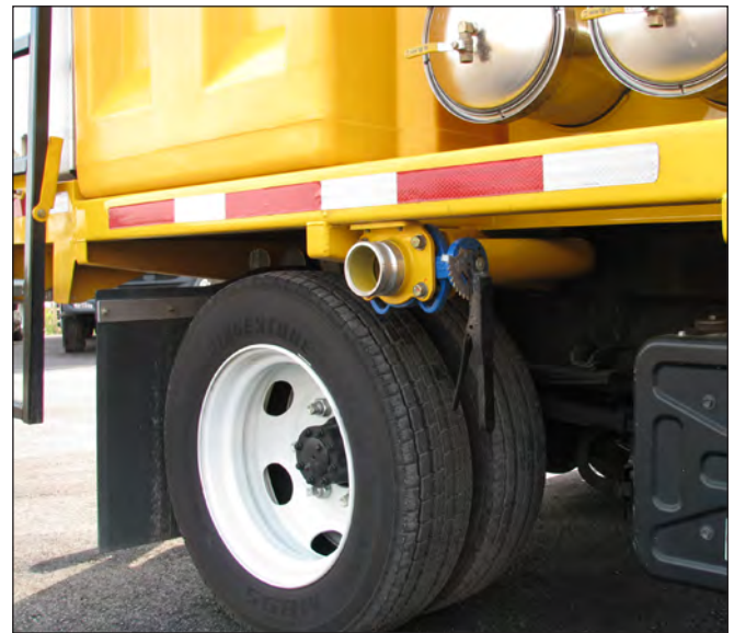
Clean Water Tank Drain Valve
