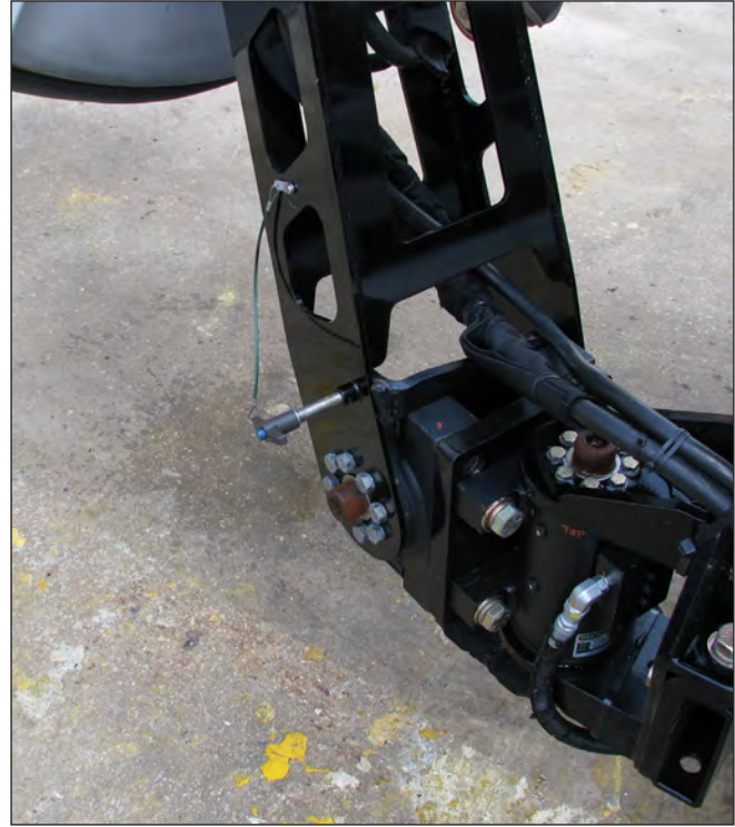
Hog Arm T-Handle Safety Pin Released & Seated In Detent Hog Arm Released & Can Be Lowered For Operation
