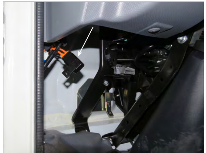
In-Line Fuse For Switch Panel Relay
