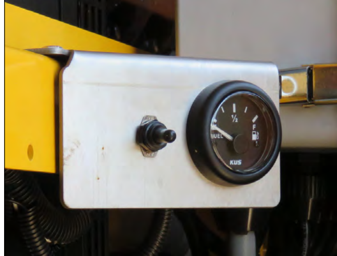
Fuel Gauge & Work Light Switch Panel
