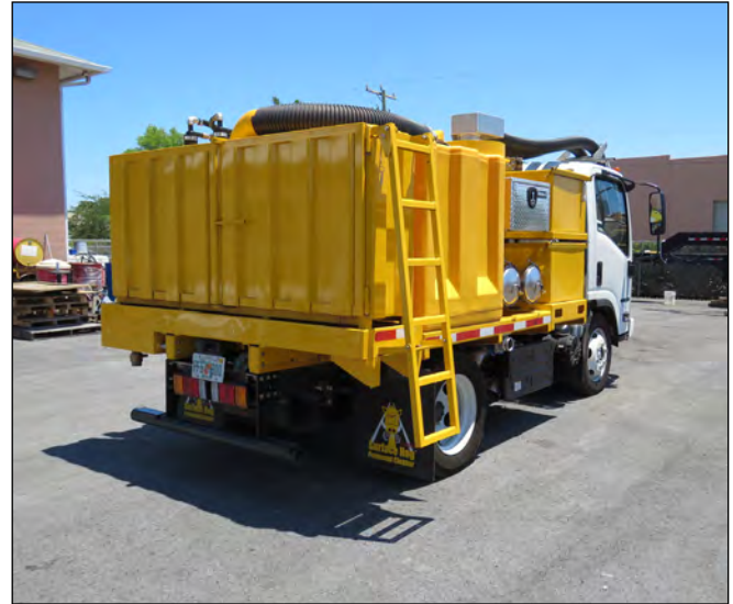
Debris Tank Ladder Deployed
