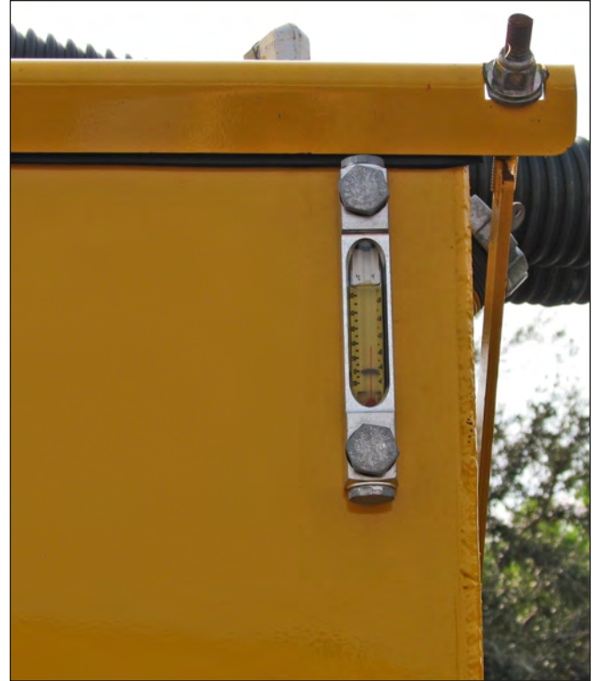
Hydraulic Tank Oil Level & Temperature Gauge
