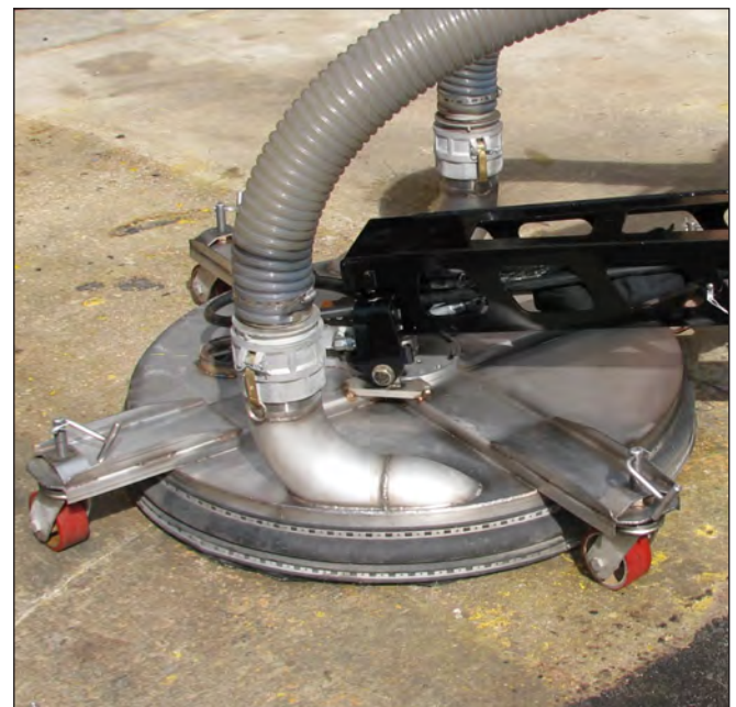
Proper Wear Brush Contact
