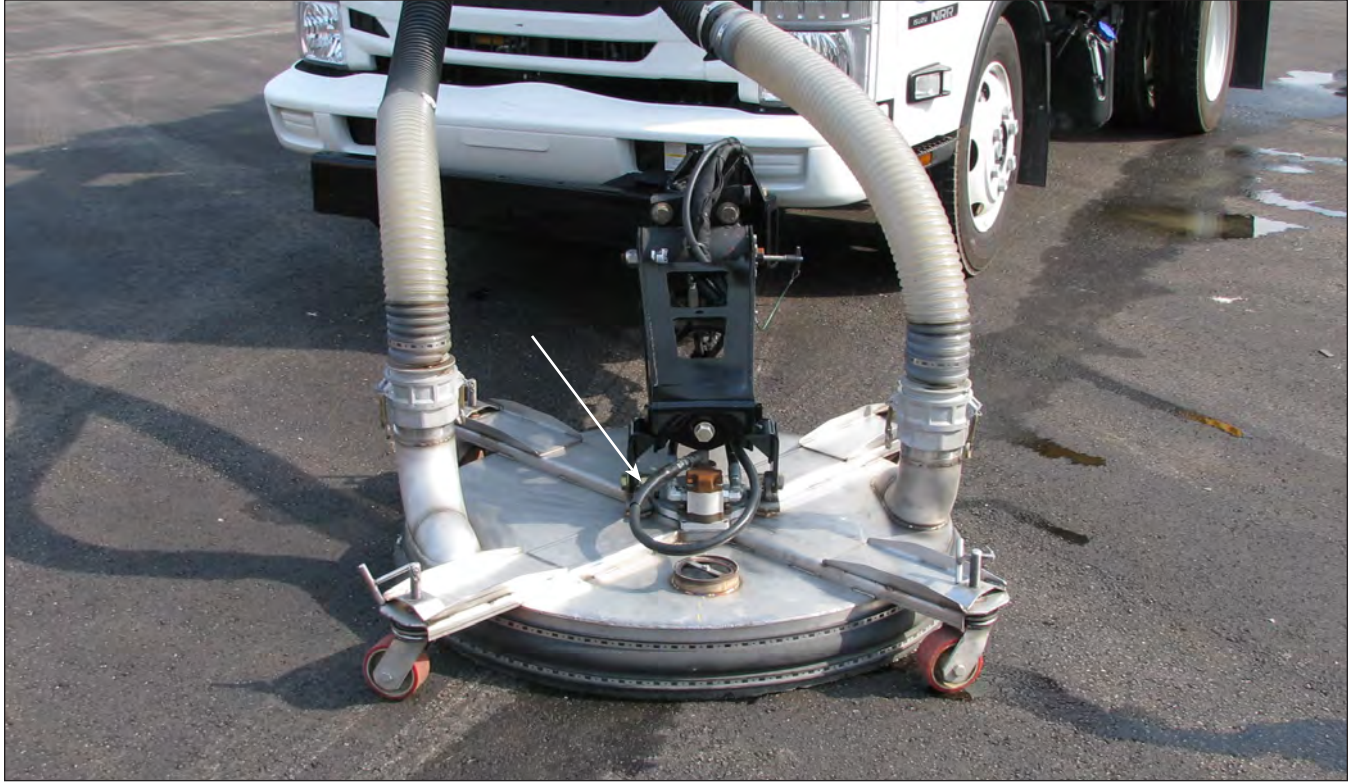
High Pressure Hose At Hog Head
