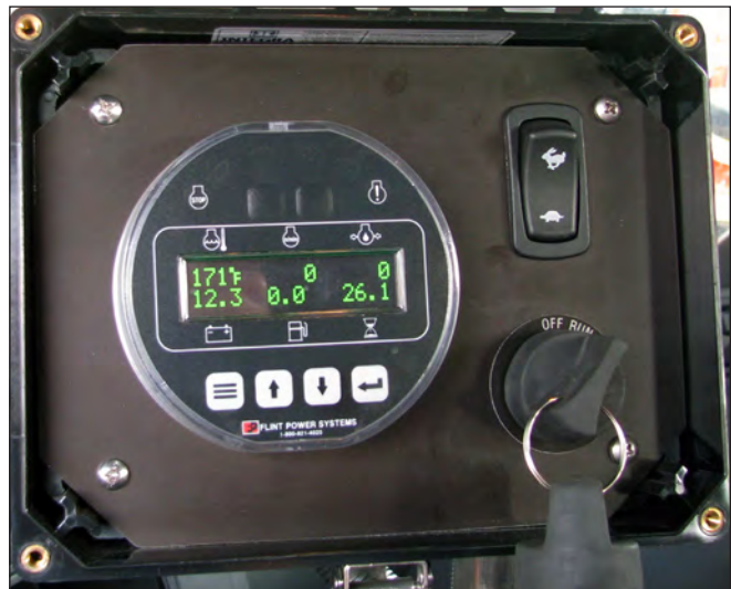
Auxiliary Engine Control Panel
