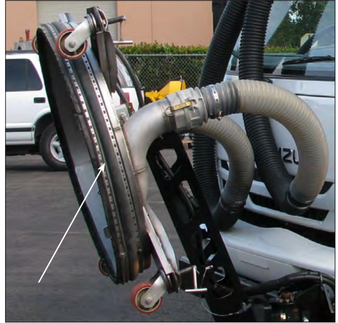
Wear Brush & Adjustment Clamps
