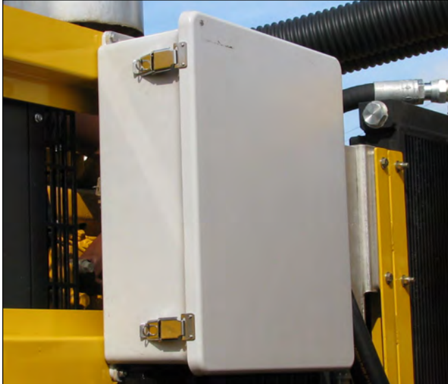
Outside Terminal Box (OTB)
