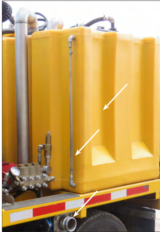
Clean Water Tank, Sight Gauge & Fill Fitting
