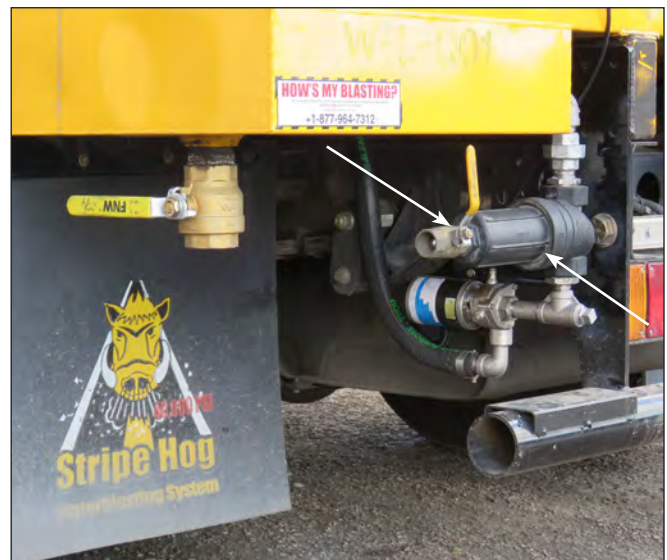
Dirty Water Pump Strainer & Drain Valve
