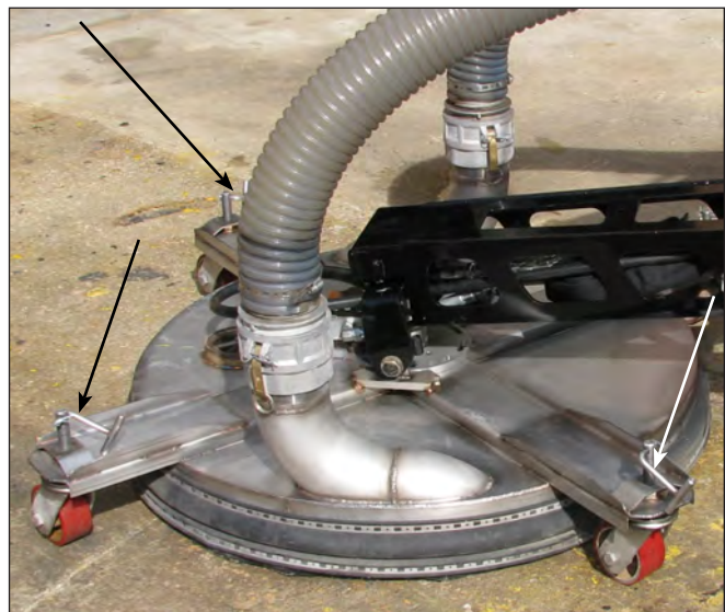
Caster Wheel Threaded Shafts & Adjustment Handles
