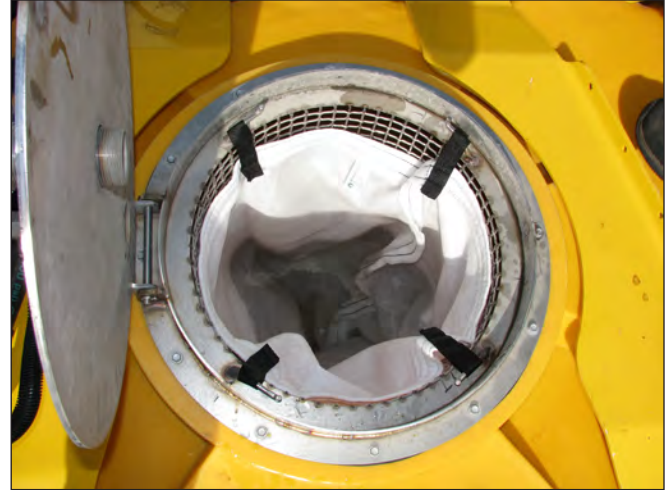
Clean Water Tank Bag Filter & Gage
