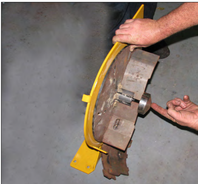
Hub Cap On Blades & Bolt Location
