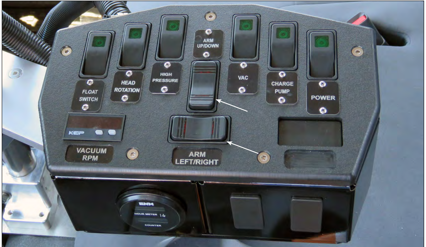
Control Switch Panel & Hog Arm RIGHT/LEFT - UP/DOWN Switches
