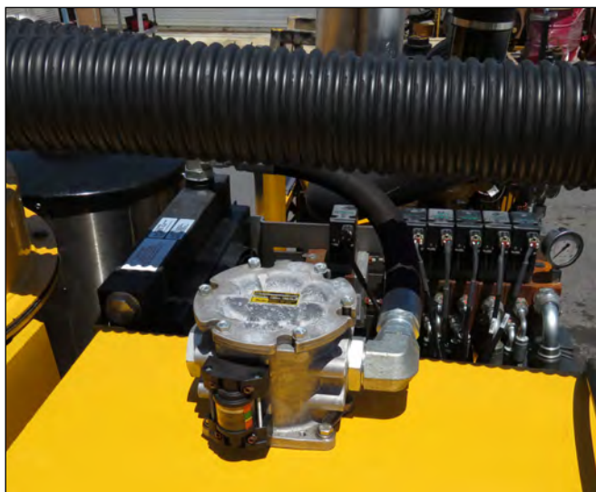
Low Pressure Hydraulic Filter
