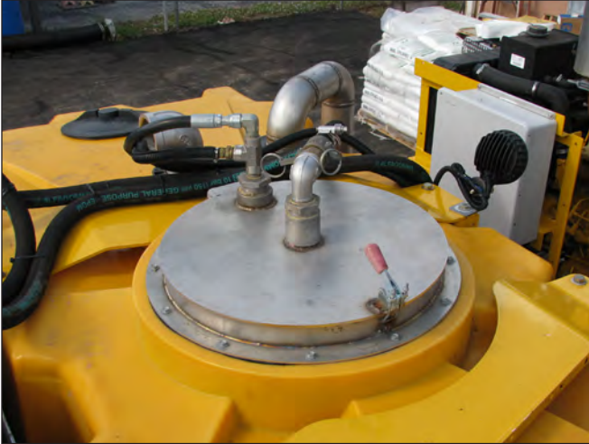
Clean Water Tank Man-Way Hatch
