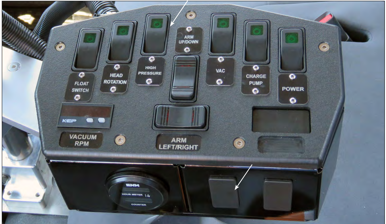
Control Switch Panel Showing High Pressure & Water Heater Switch Locations
