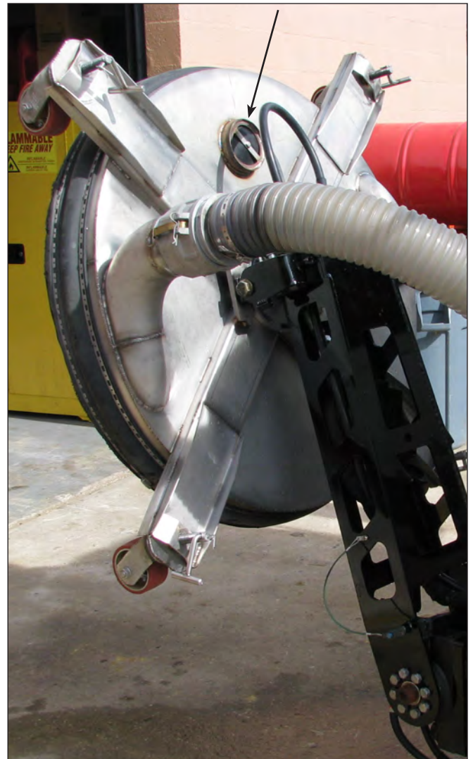
Hog Head Vacuum Check Valve
