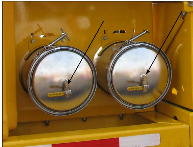
20 Micron Filter Cartridge Drain/Purge Valves
