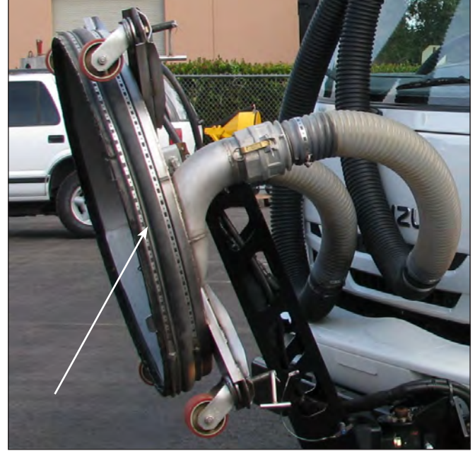
Wear Brush & adjustment Clamps
