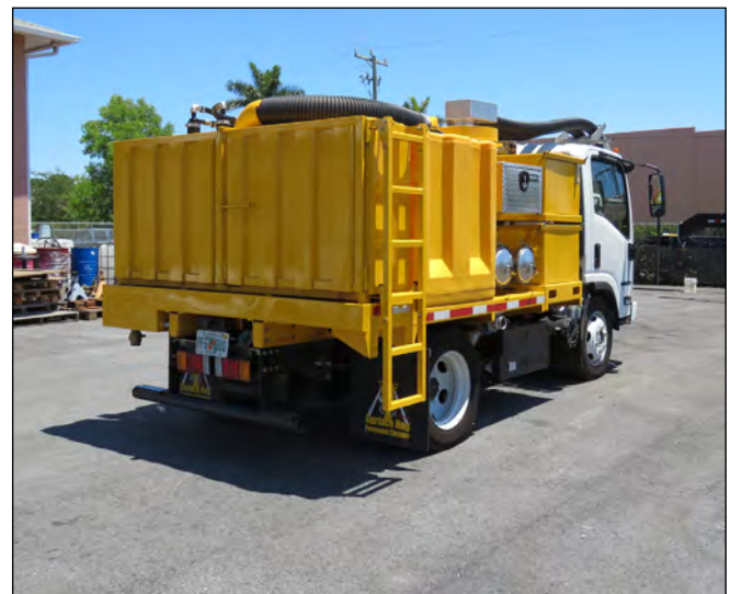
Debris Tank Ladder Stored & Secured With T-handle Safety Pin
