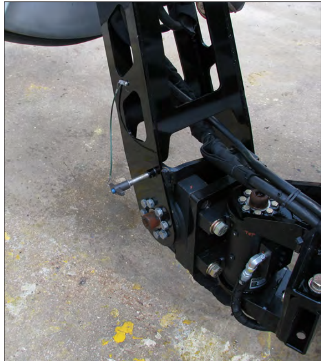
Hog Arm T-Handle Safety Pin Released & Seated In Detent
