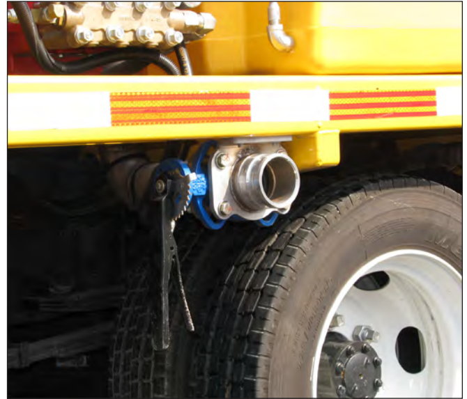
Clean Water Tank Fill Hose Connection & Valve
