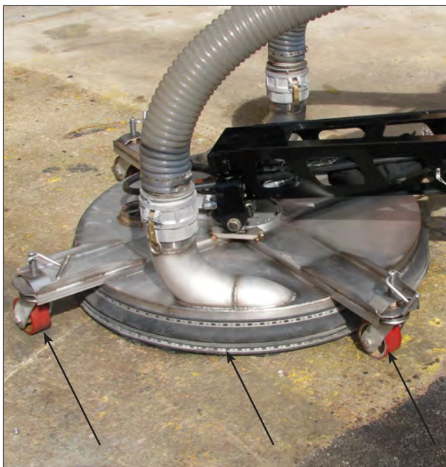
Hog Head Caster Wheels & Wear Brush
