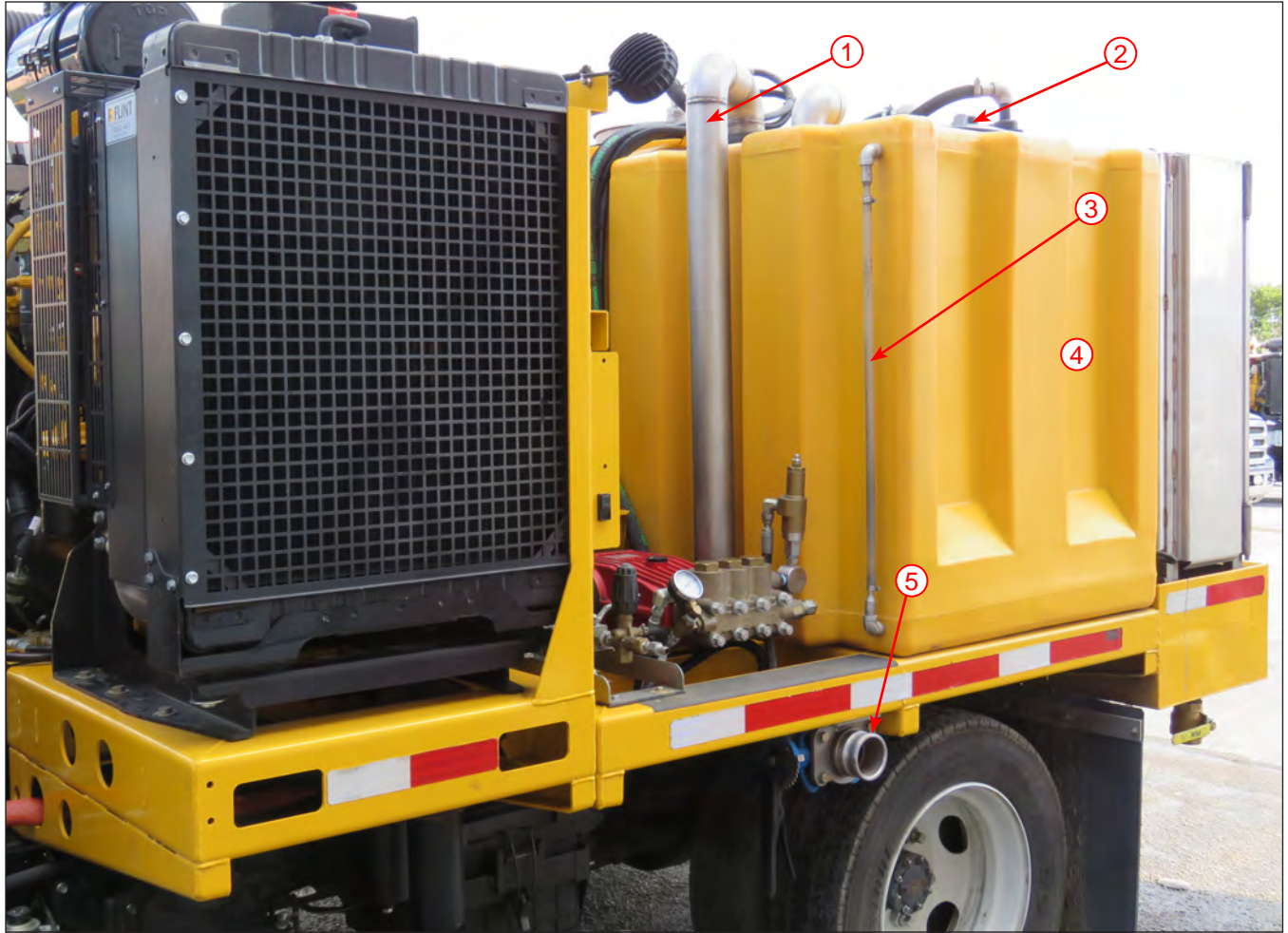
Clean Water Tank
