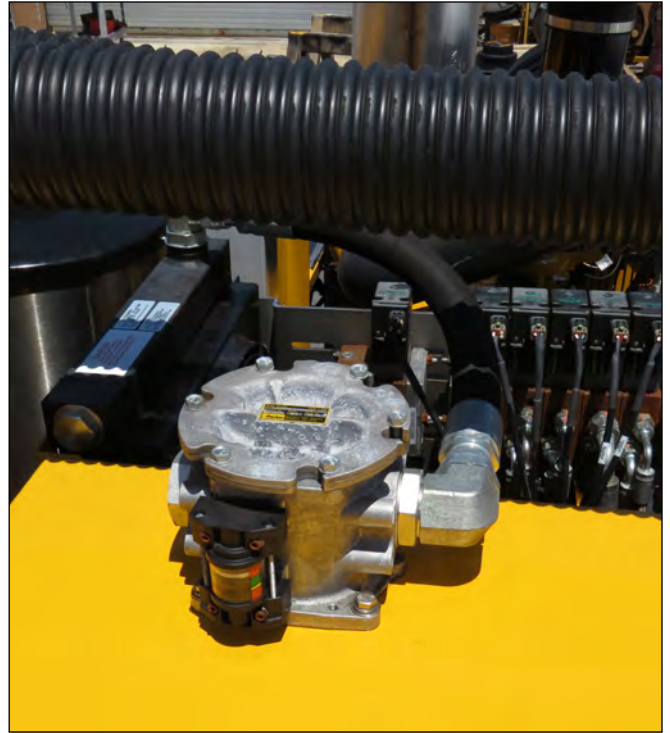
Typical Low Pressure Hydraulic Filter With Indicator Gauge
