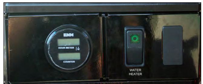
Water Heater Switch In Cab Switch Panel
