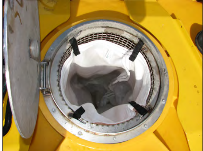
Bag Filter In Filter Cage
