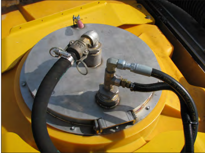
Man-Way/Water Tank Filter Access Hatch
