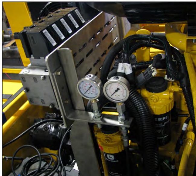
Charge Pressure & High Pressure Gauges Visible Through Cab Rear Window
