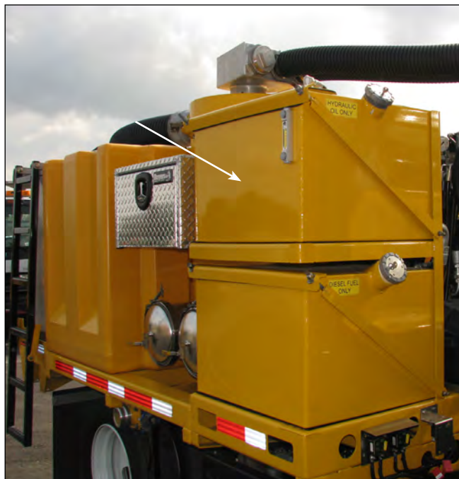
Hydraulic Fluid Tank
