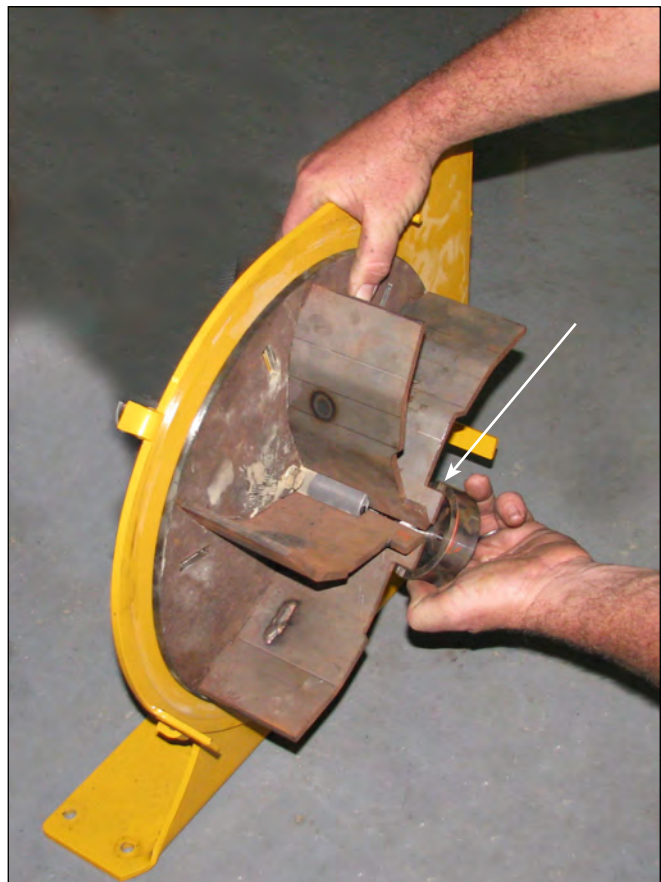
Blades Installed On Drive Plate & Hub Cap Installation
