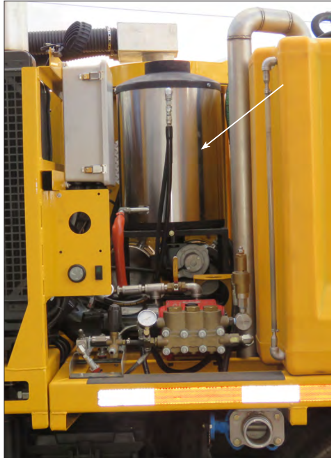
On Demand Water Heater
