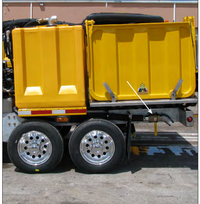
Wastewater Bladder Drain Valve
