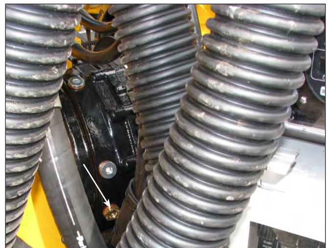
UHP Pump Reduction Gear Sight Glass
