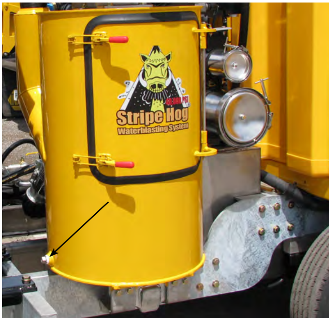
Filter Canister Drain Plug
