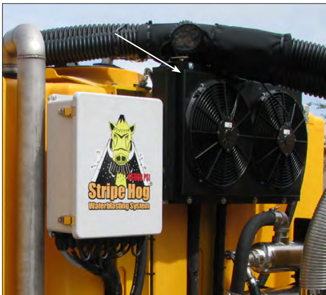
Hydraulic Fluid Heat Exchanger & Cooling Fans
