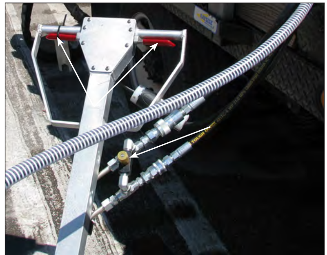
Typical Hog Tool Control Levers & Adjustable Head Rotation Speed Control Valve
