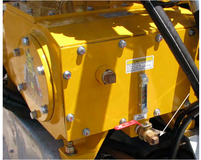
Crankcase Oil Drain Valve & Safety Plug
