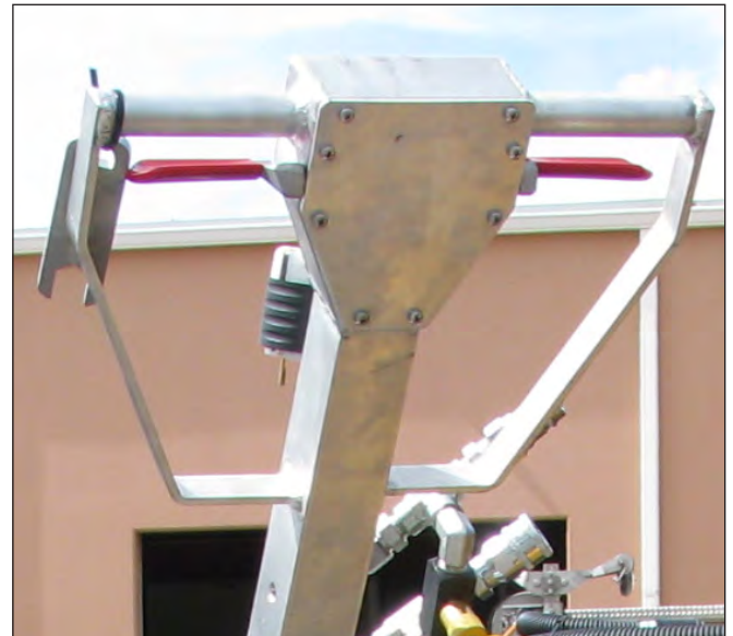
Ground Hog Spray Bar Rotation & UHP Control Levers
