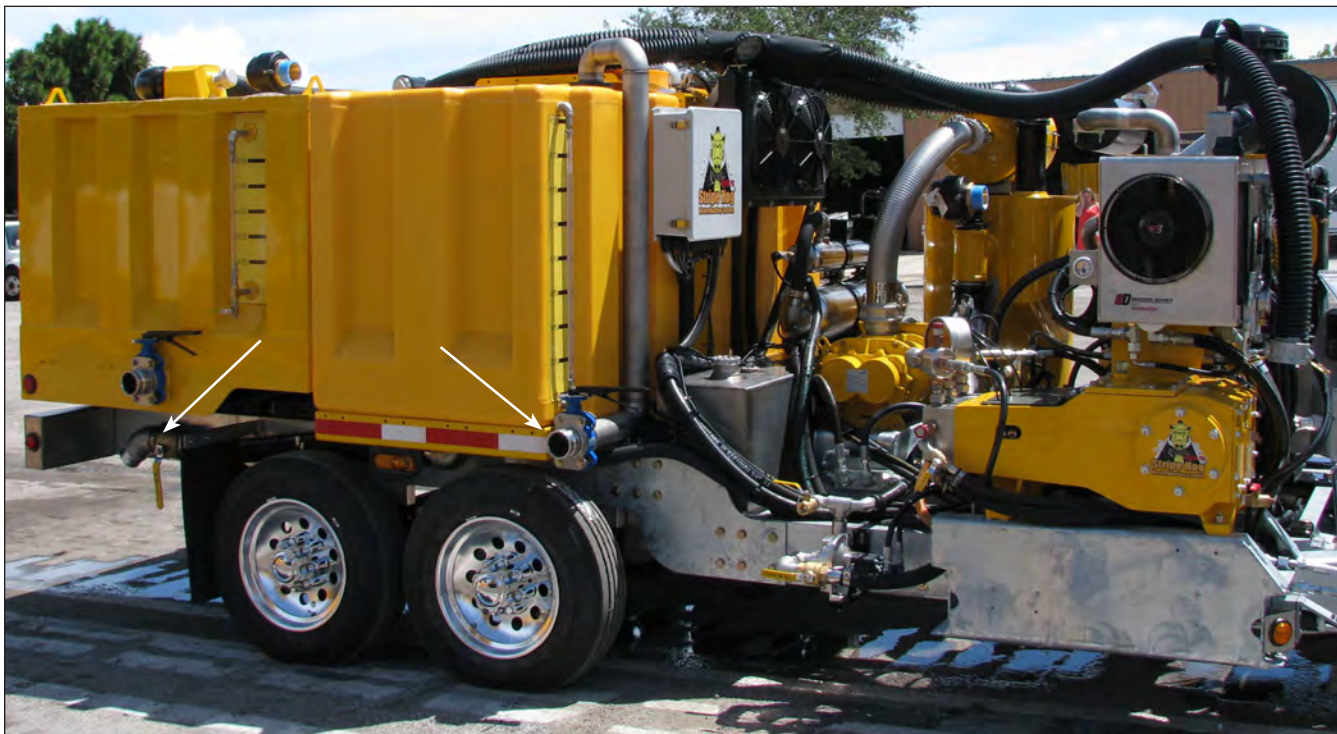
Clean Water Tank Drain & Fill Valves
