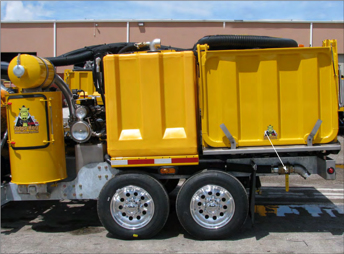
Wastewater Bladder Drain Valve
