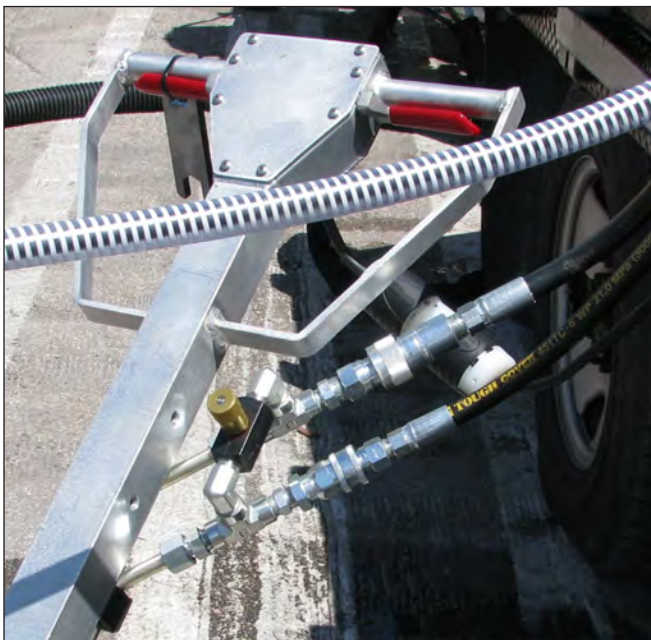
Ground Hog Spray Bar Rotation Control Valve
