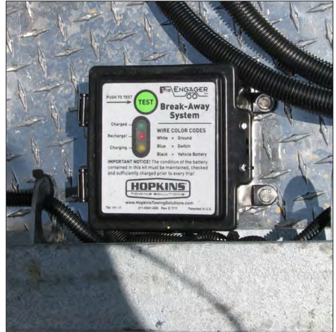
Trailer Break-Away System & Battery
