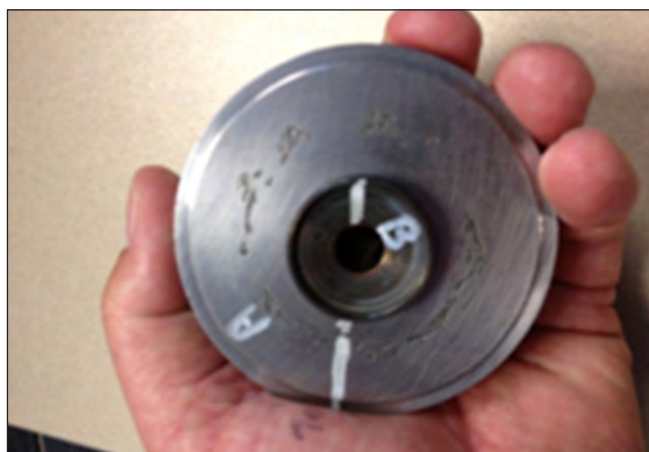
Figure 3: A. Univalve Body - B. Suction Valve Suction Valve Rotated 90° Clockwise
