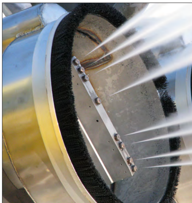
Nozzle Pressure Test - All Nozzles Good
