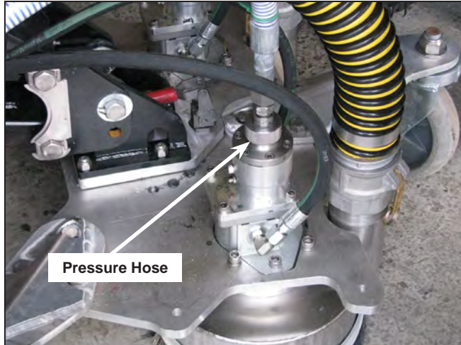
Figure 1: High pressure hose on top of the thru-shaft motor
