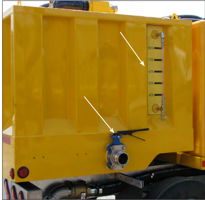
Debris Tank Drain Valve & Water Level Sight Gauge
