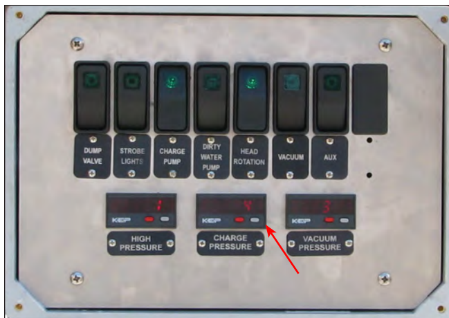
Digital Charge Water Pressure Gauge In Switch Panel
