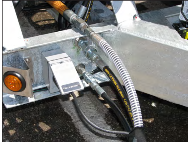
Hog Tool Control Harness, Hydraulic Hose Quick Disconnect Fittings & High Pressure Hose Connection
