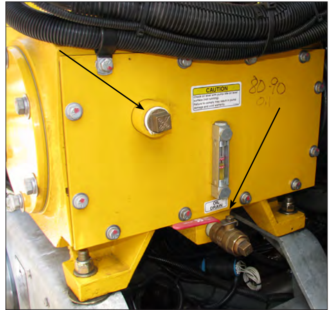
Back Plate Fill Port - Preferred Oil Fill Location Crankcase Oil Drain Valve
