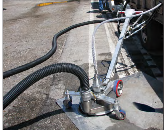
Ground Hog With All Hoses & 12V Control Cord Connected
