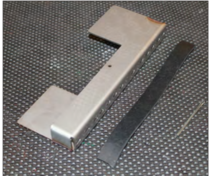
Spray Bar Protector, Cotter Pin & Gasket
