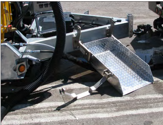
Ground Hog Landing Pad Lowered To Pavement & Tie Down Strap
