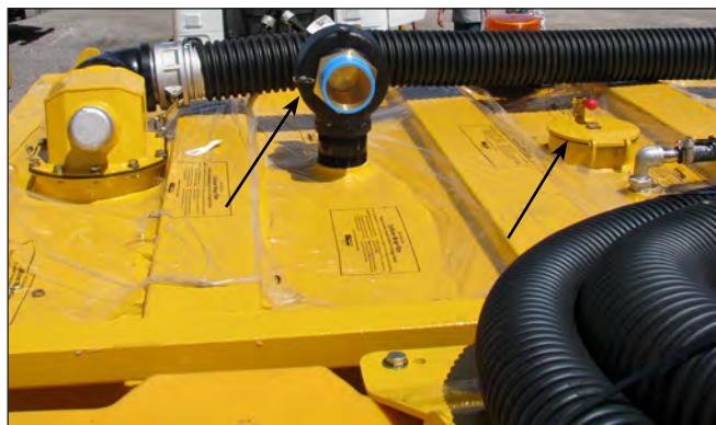
Vacuum Tank Kunkle Valve & Inspection Port
