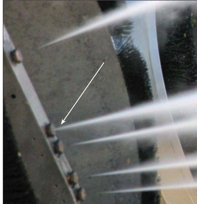
Nozzles Showing Bad Spray Pattern Nozzle Must Be Replaced
