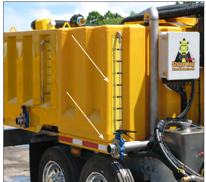
Clean Water Tank Fill Hose Connection Valve & Site Gauge
