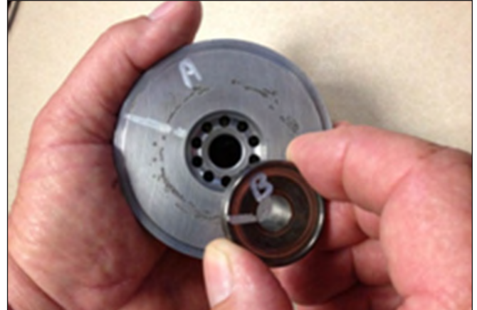
Figure 1: A. Univalve Body & Seat - B. Suction Valve
