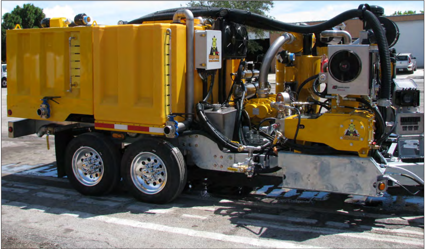
SK2000 Water Blasting System Mounted On A Trailer Chassis
