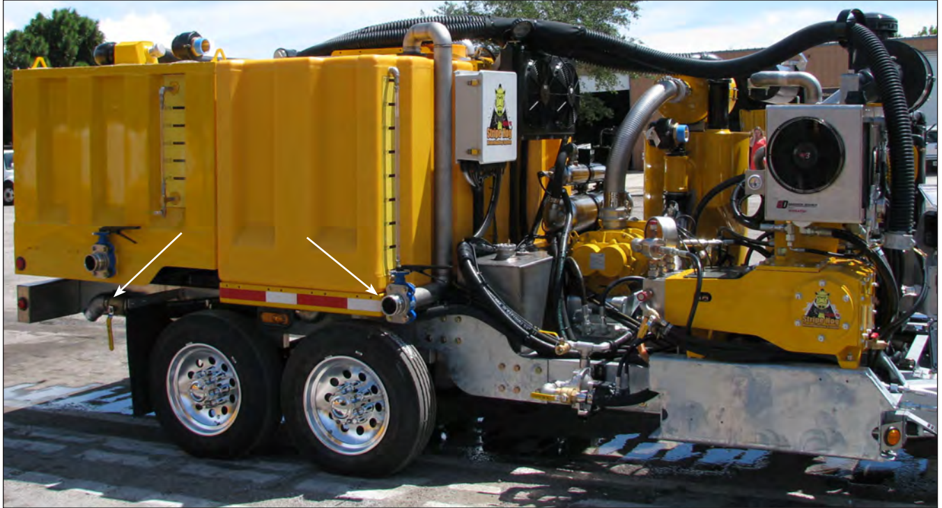
Clean Water Tank Drain & Fill Valves
