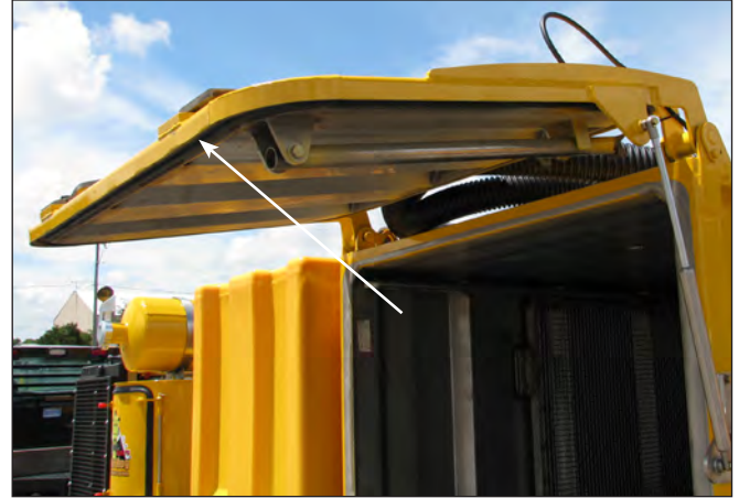
Debris Tank Inflatable Door Seal
