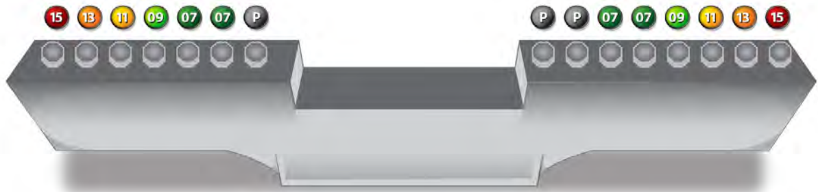
13) 14" Most Aggressive set-up. 5.66 GPM @ 36K psi / 5.98 GPM @ 40K psi .....
