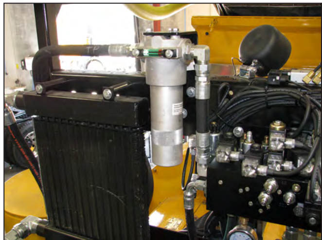
Hydraulic System Oil Cooler with Thermostatically Controlled Fan, In-Line Filter and Filter Change Indicator
