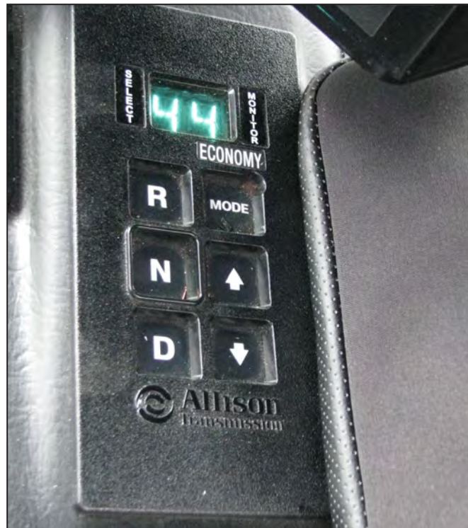
Work Mode Gears Selected with Mode Switch
