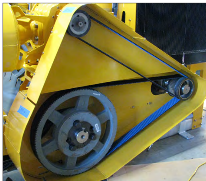
Typical Drive Belt Configuration for PTO Clutch Powered UHP Pump and Vacuum Blower
