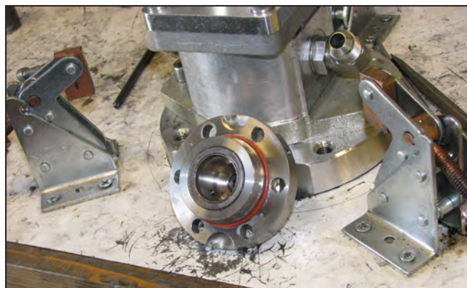
Figure 6: Thrust housing cap removed. Note the O-ring seal and the slots for the screwdrivers. Make sure the cap and O-ring is in good condition and clean.
