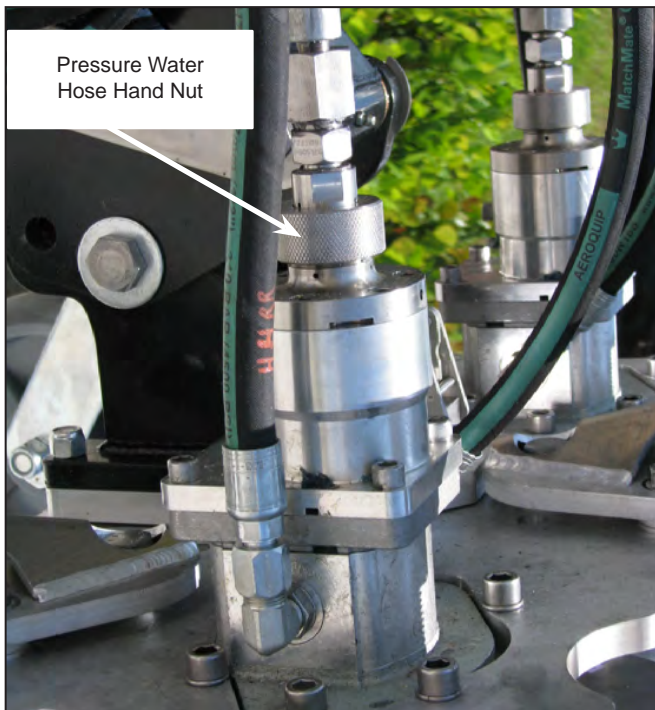
Figure 17: Apply anti-seize to the thrust housing threads and install the high pressure water line.
