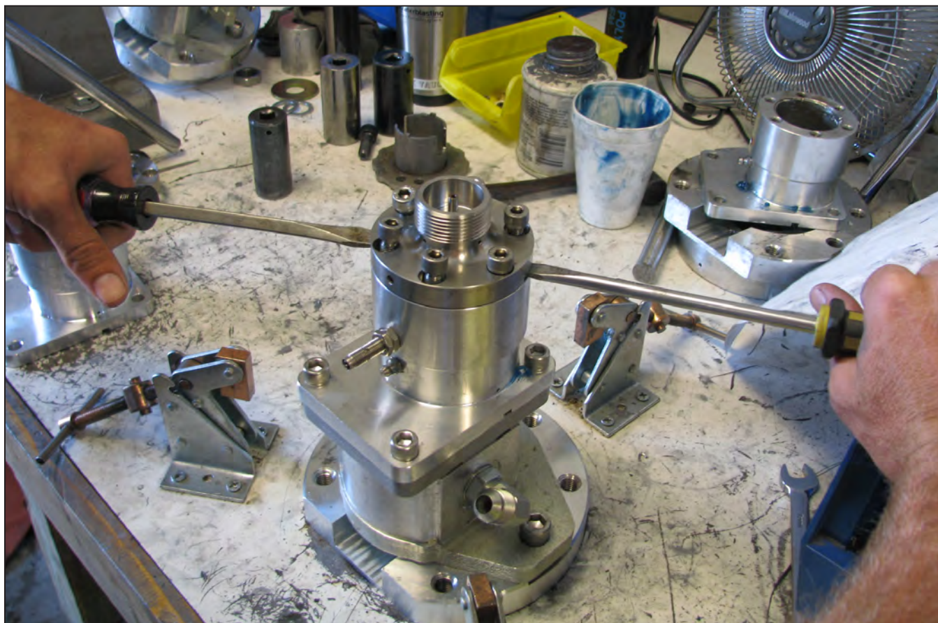
Figure 5: Use two medium flat head screwdrivers to remove the thrust housing cap. Note that the bolts are loose and left in place to prevent thrust housing cap from falling and being damaged during removal.
