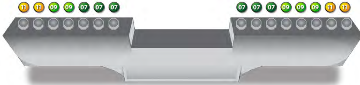
15) 14" Least Aggressive set-up. 4.81 GPM @ 36K psi / 5.09 GPM @ 40K psi .....
