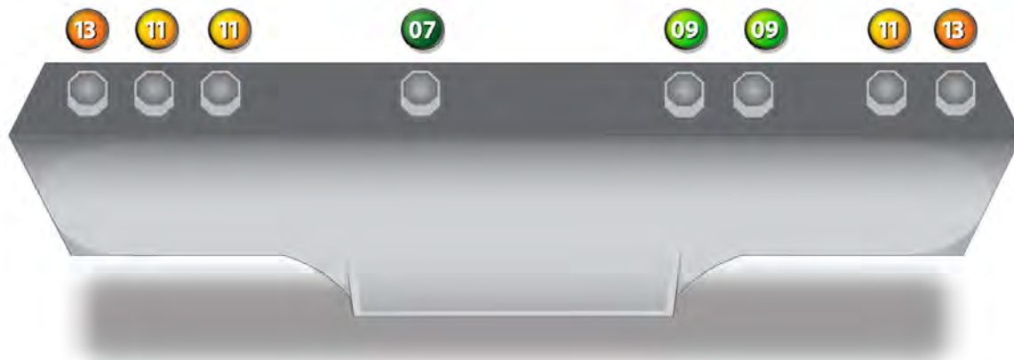
4) 8", 8 Nozzle -Least Aggressive set-up. | 3.71 GPM @ 36K psi | 3.93 GPM @ 40K psi
