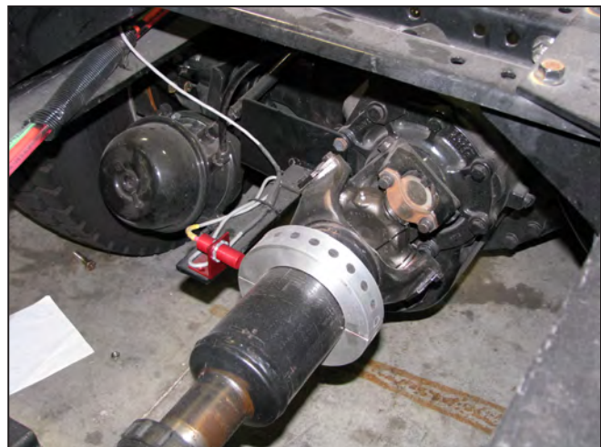
Skip Meter Inductive Pickup on Drive Shaft
