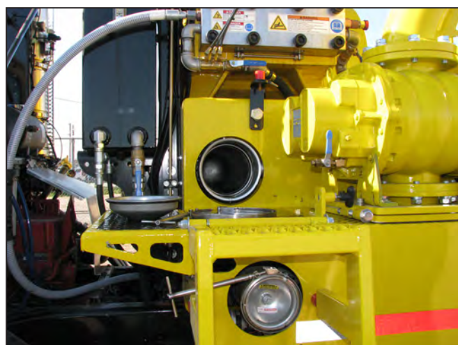
Charge Water Filters Top Filter is 10 Micron (Nominal) Bag Type Filter Bottom is 1 Micron (Absolute) Cartridge Type Filter
