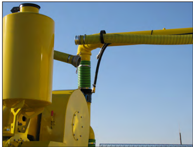
Disconnect Hoses at Quick Disconnect Fittings Before Dumping
