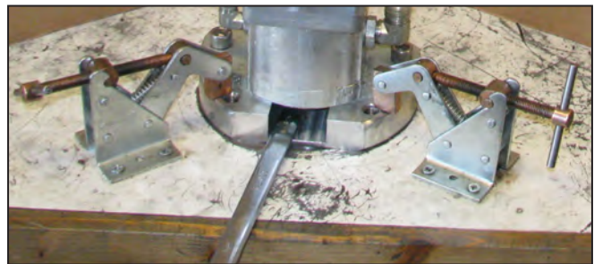
Figure 8: 3/4" (19mm) open end wrench holding thru-shaft and preventing it from turning while removing swivel tit assembly/gland nut.
