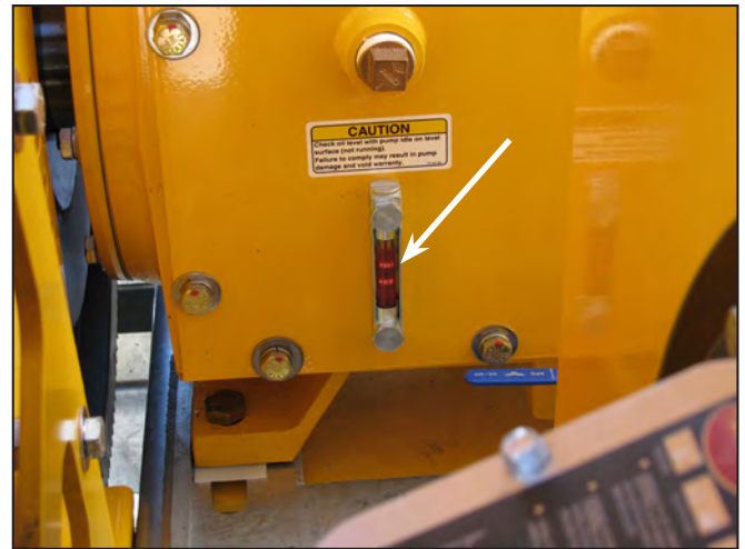
UHP Pump Oil Sump Level Indicator and Oil Fill
