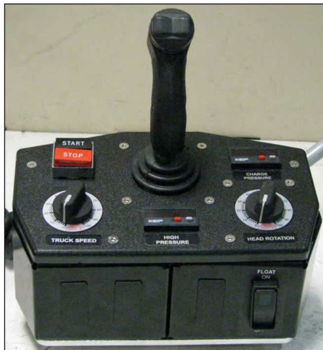
Joystick Control Panel with Speed Dials, Pressure Gauges, UHP Switch and Float Mode Switch
