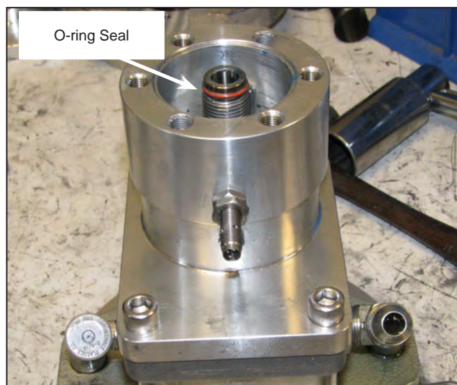
Figure 13: O-ring seal at the top of the thru-shaft greased and the threads below the seal coated with anti-seize.
