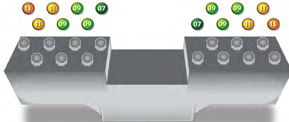
6) 6" 14 Nozzle Spray Bar - 4" lines - Argessive. | 5.72 GPM @ 36K psi | 6.0 GPM @ 36K psi
