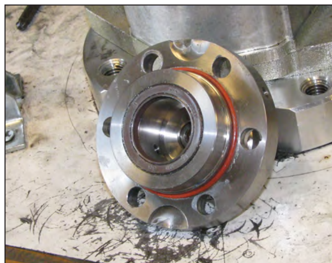
Figure 15: Inspect and grease the O-ring seal on the thrust housing cap.
