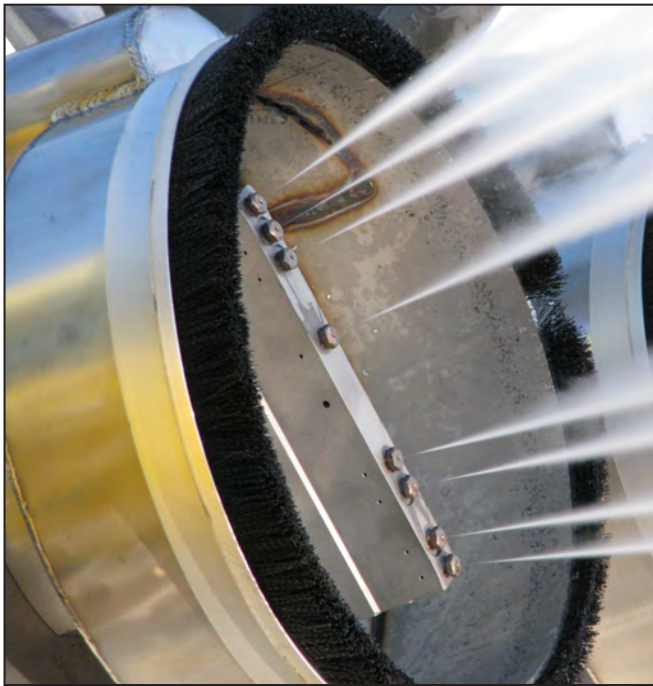
Good Nozzle Spray Pattern and No Water at Weep Holes
