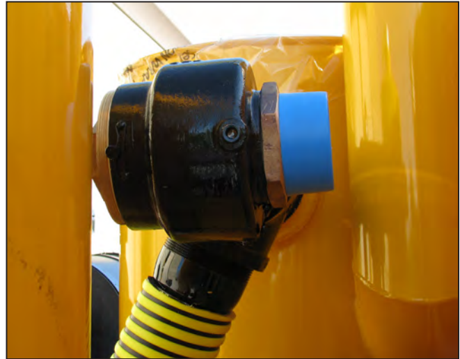
Vacuum Relief Valve (Kunkle Valve) on Vacuum Filter Canister
