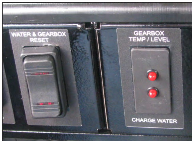
Water & Gearbox Reset Switch Gearbox Temp/Level & Charge Water Warning Lights
