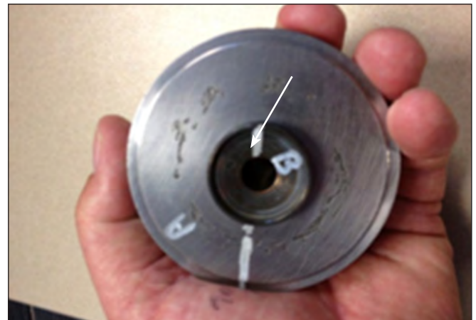
Figure 3: A. Univalve Body - B. Suction Valve Suction Valve Rotated 90° Clockwise
