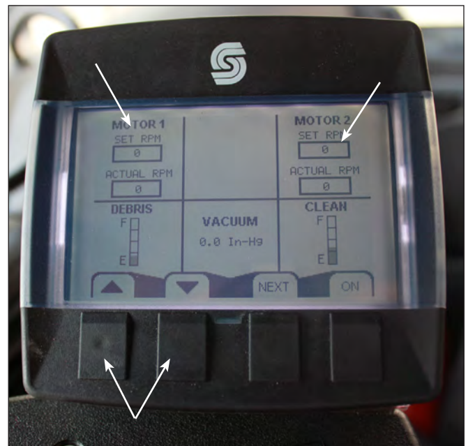
Main Screen Display Showing Controls, Spray Head RPM, Debris & Clean Water Tank Levels & Vacuum Pressure
