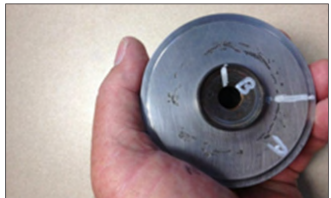
Figure 4: A. Univalve Body - B. Suction Valve Valve Cartridge Rotated 90° Clockwise
