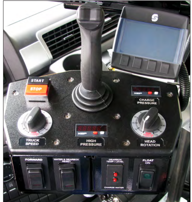
Joystick Control Console With Forward/Reverse Switch, Truck Speed Dial, Head Rotation Speed Dial, START/STOP Buttons, Float Switch, Charge Water Pressure Gauge, UHP Pump Water Pressure Gauge, Joystick & PLC
