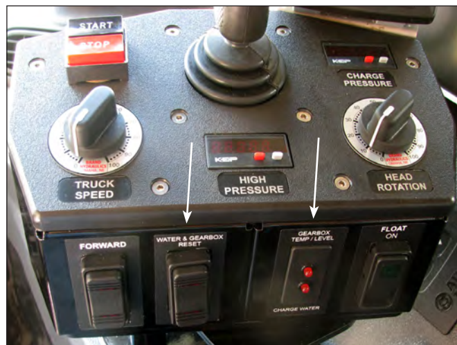
Water & Gearbox Reset Switch Temp/Level/Charge Water Cutout Indicator Lights
