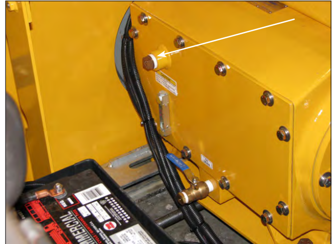
Back Plate Fill Port - Preferred Oil Fill Location
