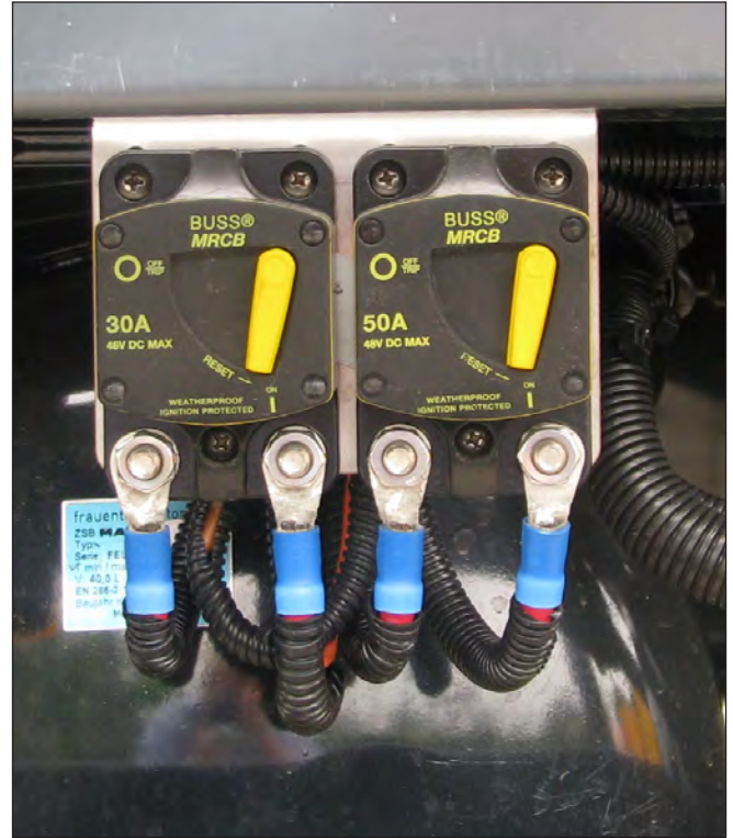
Typical 50 AMP & 30 Amp Main Fuses That Protect Waterblasting Electrical System
