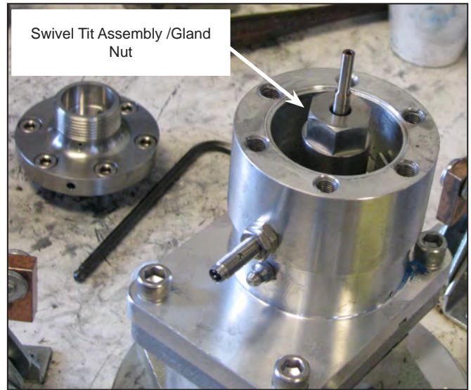
Figure 14: Swivel tit assembly/gland nut installed on the thru-shaft and torqued to 50 Ft lbs.
