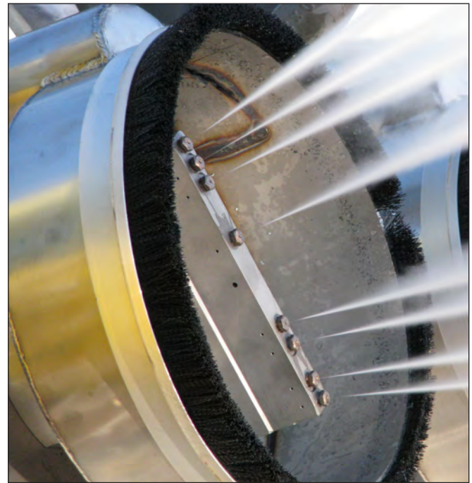
Nozzle Pressure Test - All Nozzles Good
