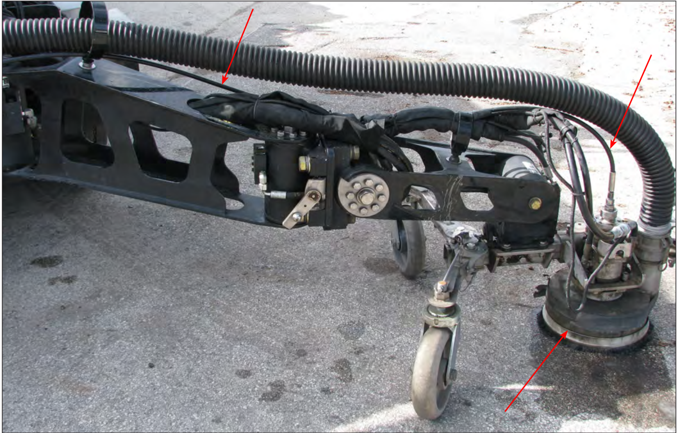
Blasting Head & Ultra-High Pressure Hose
