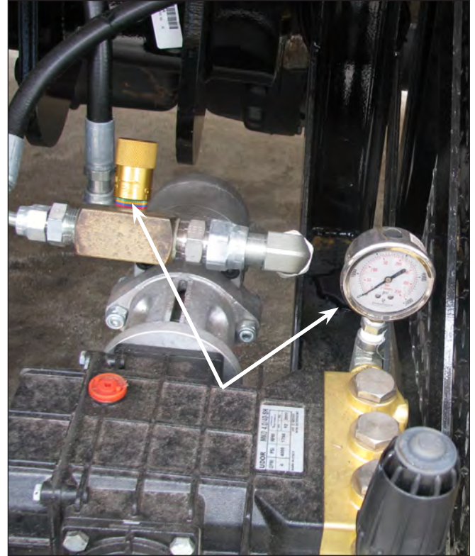
Hydraulic Pressure Valve Set To Green Ring Water Pressure Gauge
