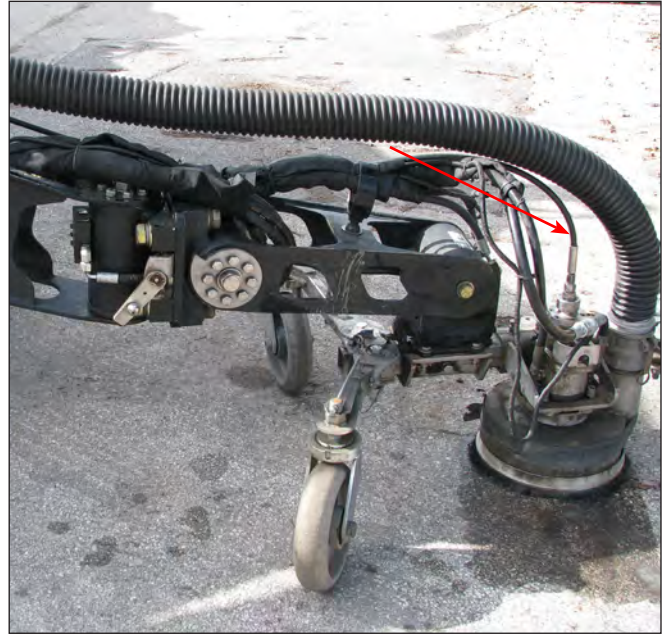
Typical High Pressure Water Hose
