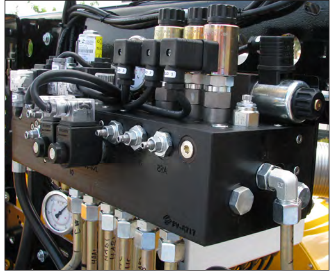
Hydraulic Manifold, Solenoid Valves & Gauges
