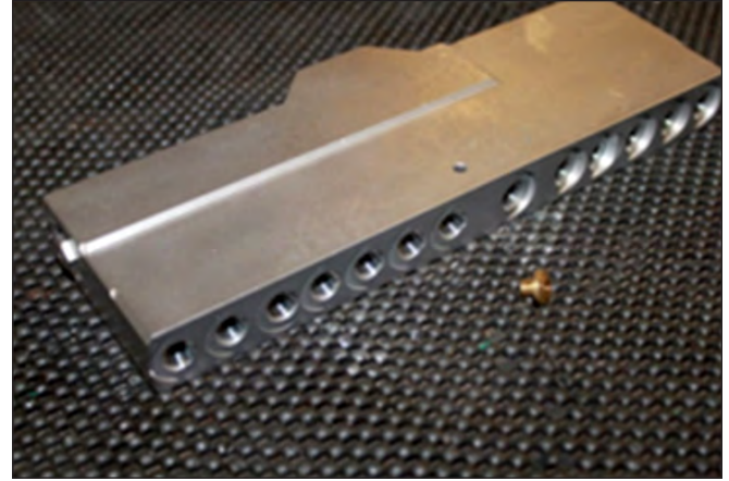
Typical Spray Bar & Nozzle
