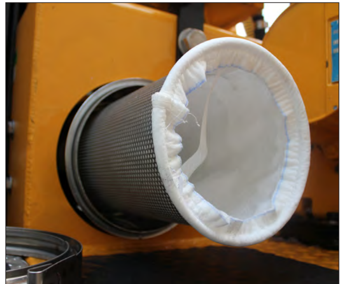
Typical 10 Micron Bag Style Filter
