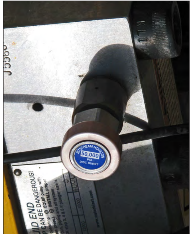
Typical 50,000 PSI (3,448 BAR) Rupture Disc On UHP Manifold
