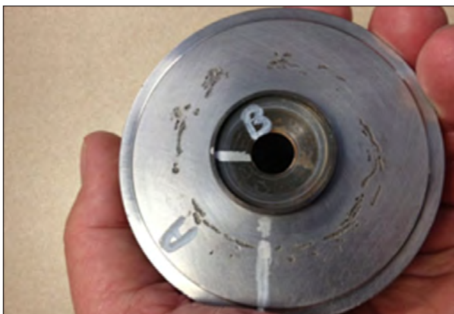
Figure 2: A. Univalve Body - B. Suction Valve Valve Cartridge Rotated 90° Counterclockwise
