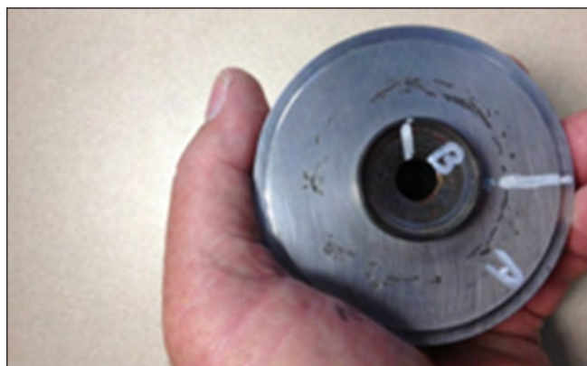
Figure 4: A. Univalve Body - B. Suction Valve Valve Cartridge Rotated 90° Clockwise
