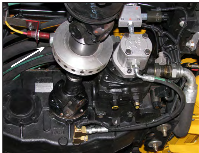
Typical Skip Meter Inductive Pickup On Drive Shaft
