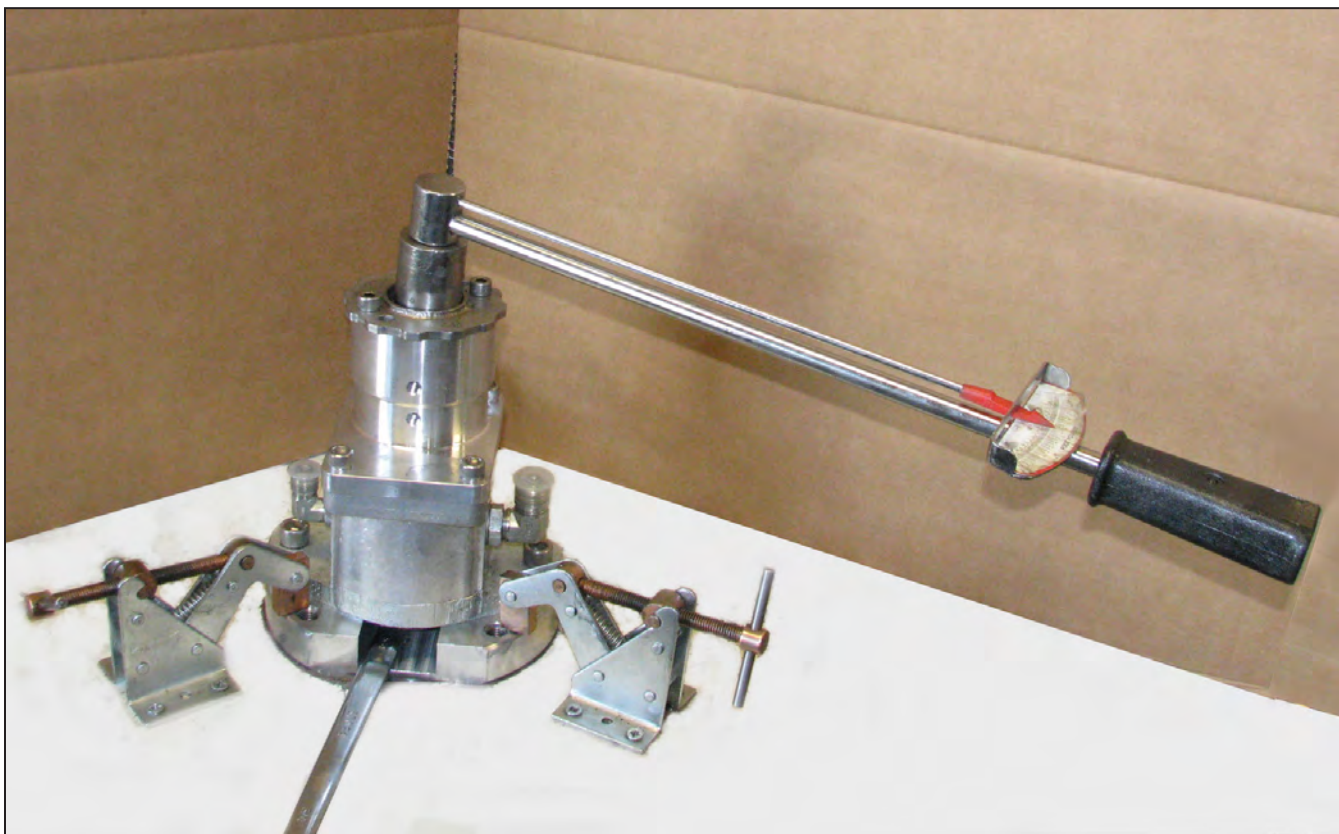
Figure 12: Thrust housing cap bolts securing the spanner tool are snug and a torque wrench and 1 1/8" deep well socket is used to tighten the jam nut to 50 Ft lbs.
