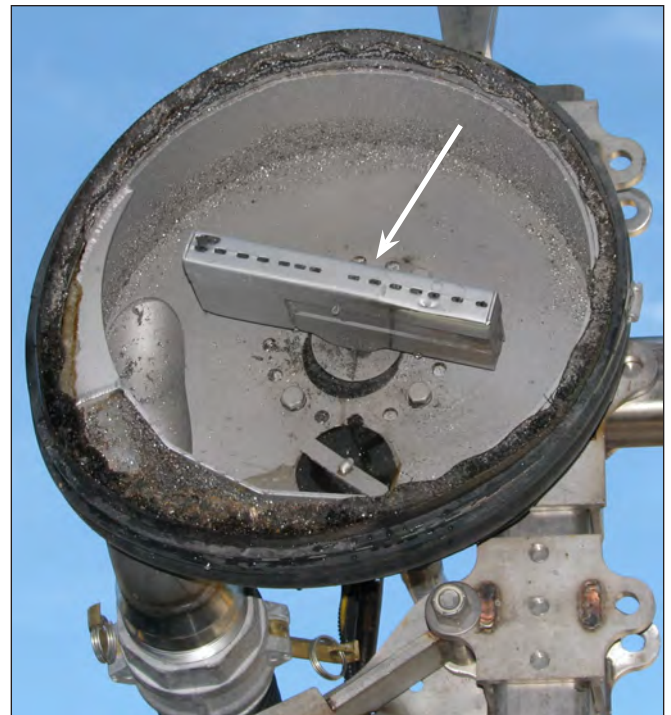
Blasting Head With Spray Bar Protector Installed
