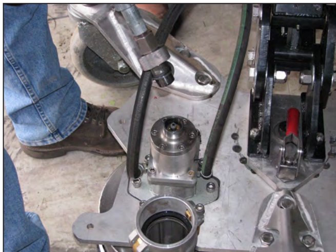
Figure 2: High pressure hose removed
