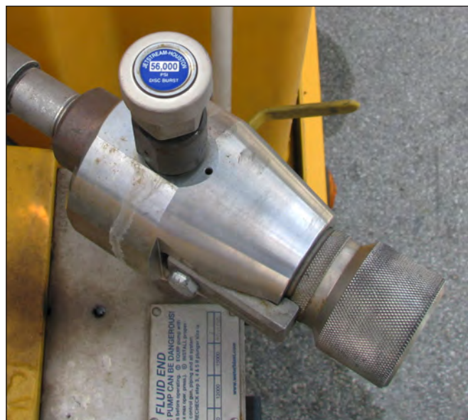
Typical Rupture Disc On Manual By-Pass Valve
