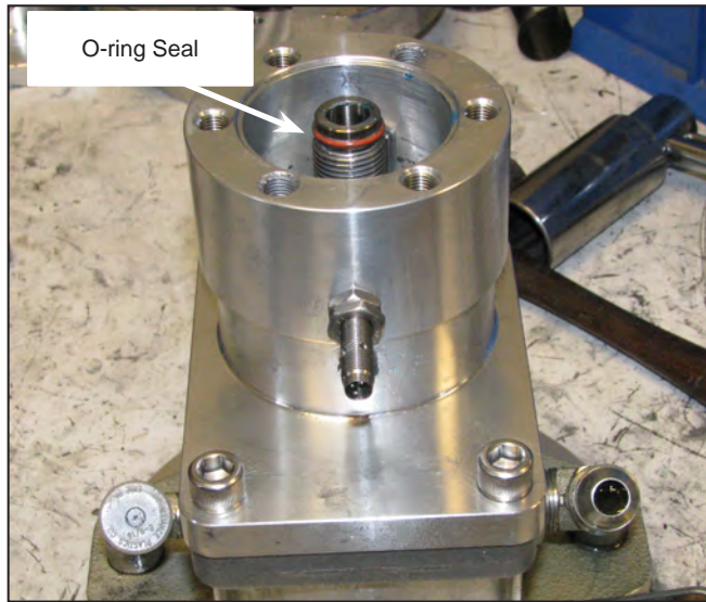
Figure 13: O-ring seal seat at the top of the thru-shaft greased and the threads below the seal coated with anti-seize.
