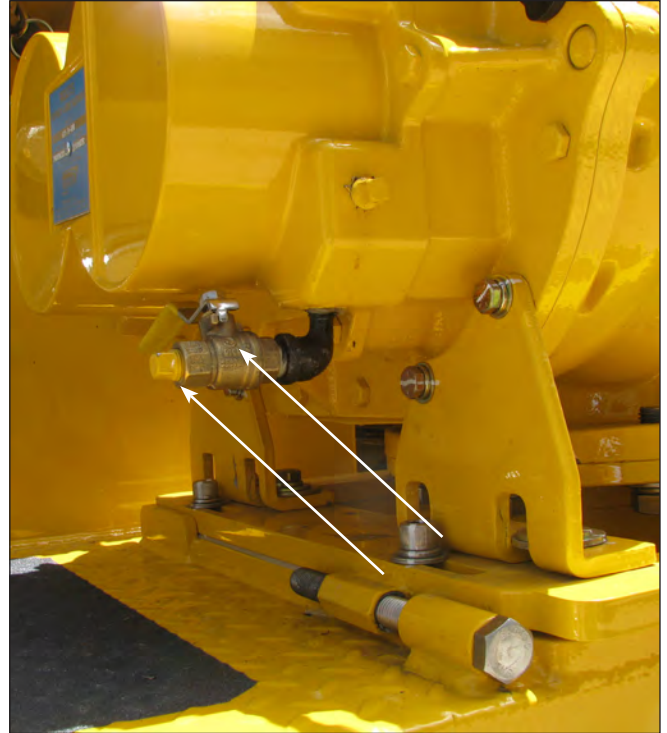
Typical Vacuum Blower Drain Valve & Safety Drain Plug
