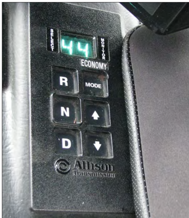
Automatic Transmission Gear Selector & LED Screen PTO Switch ON & 4/4 Lockup Displayed
