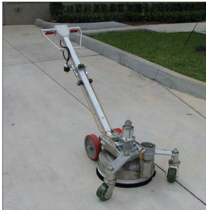
Ground Hog/Walk Behind Auxiliary Blasting Tool
