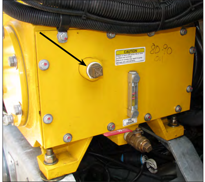
Back Plate Fill Port - Preferred Oil Fill Location
