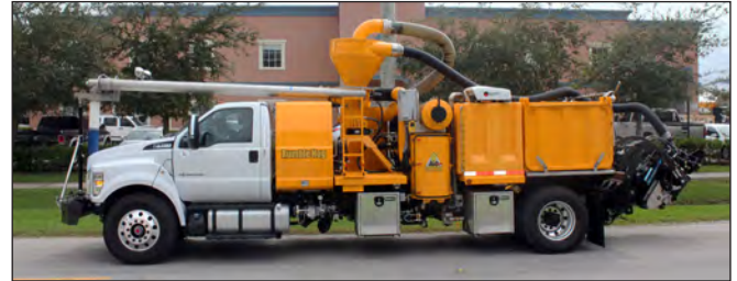
Debris Recovery System With Optional Continuous Off-Loading System
