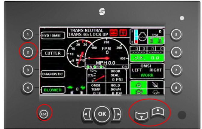
Controller MAIN Screen - Setting Down Pressure & Select Cutter Setup Screen
