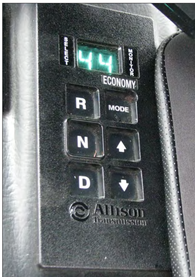
Automatic Transmission Gear Selector & LED Screen PTO Switch ON & 4/4 Lockup Displayed
