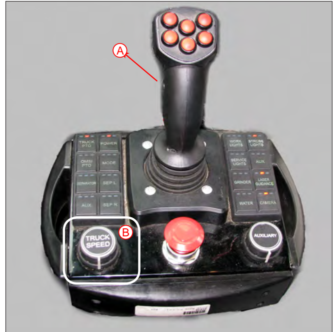
Joystick, Joystick Trigger (A) & TRUCK SPEED Dial (B)
