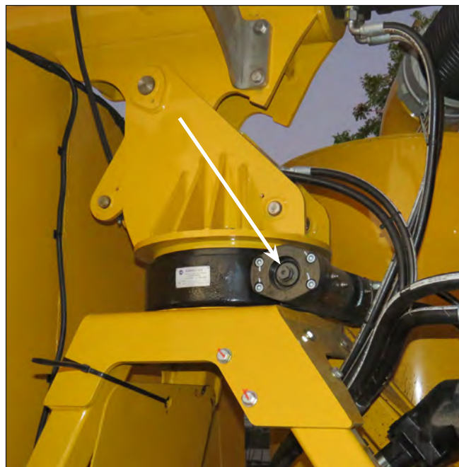
Hex Nut On Worm Gear Shaft For Manual Movement
