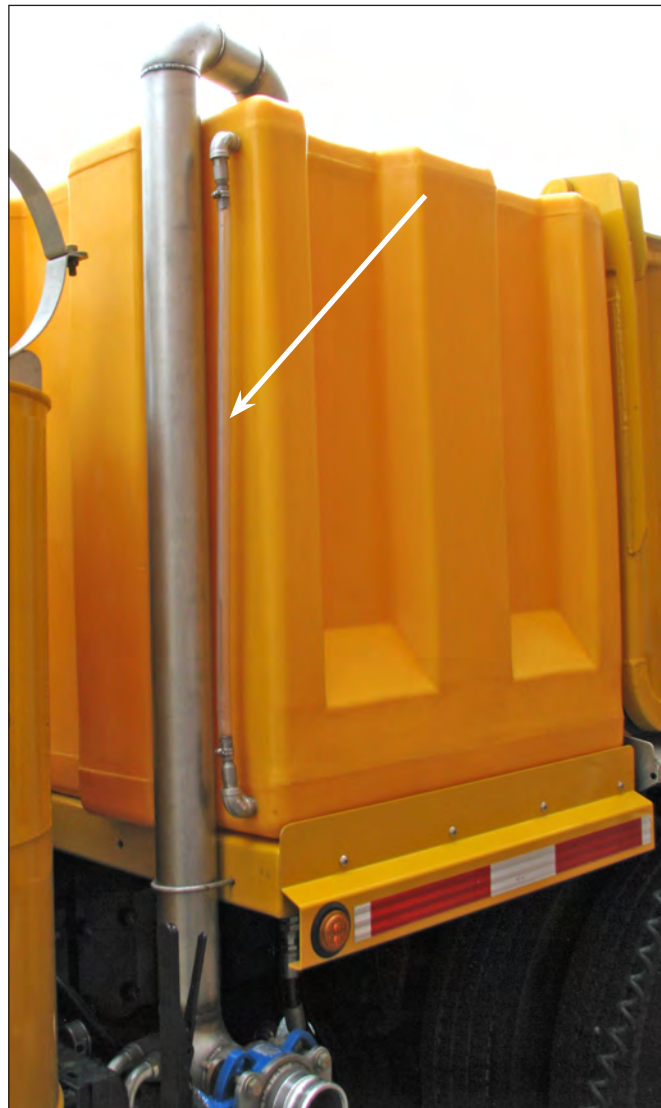
Clean Water Tank Sight Gauge
