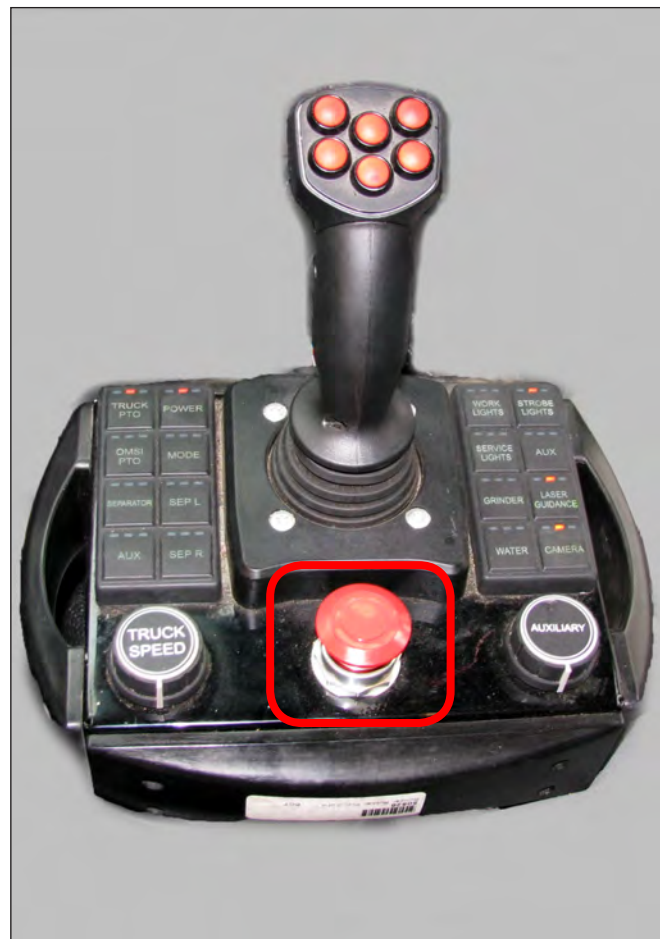
Joystick Emergency (E-STOP) Switch
