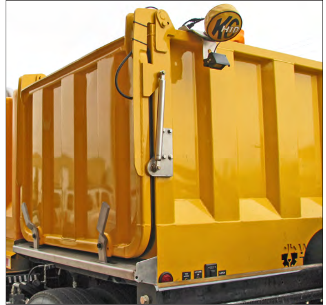
Debris Tank & Debris Tank Door
