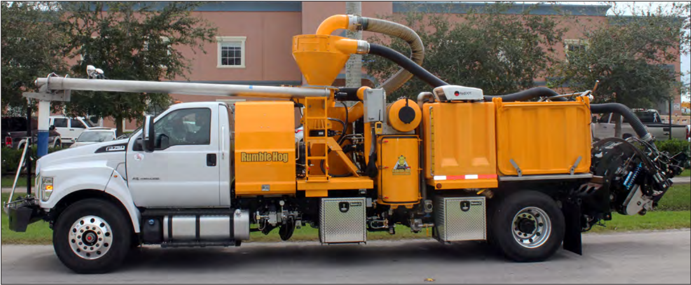
Debris Recovery System With Optional Continuous Off-Loading System
