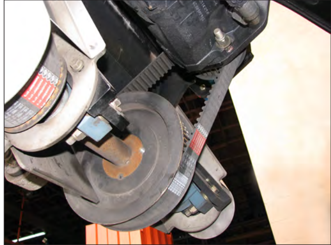
Eccentric Hydraulic Motor To Eccentric Drive Axle Belt
