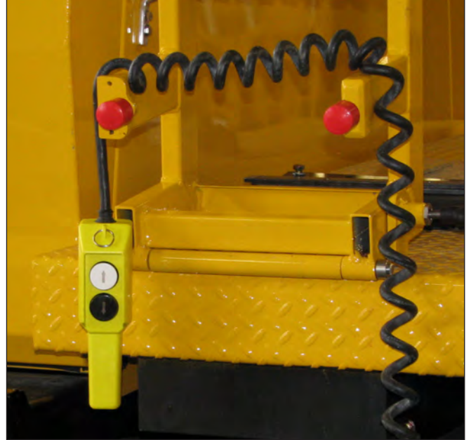
Remote Switch Control
