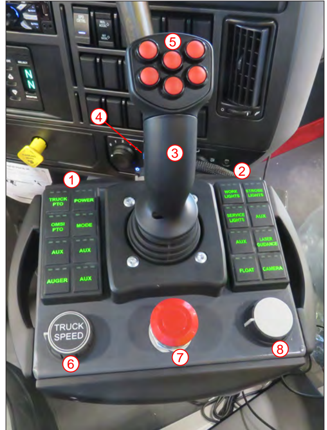
Joystick, Joystick Panels, Speed Dials & Emergency Stop Switch
