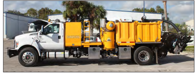
Debris Recovery System Without Optional Continuous Off-Loading System
