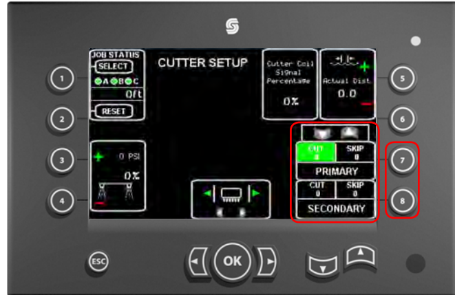
CUTTER SETUP Screen - Setting Primary & Secondary Skip Pattern
