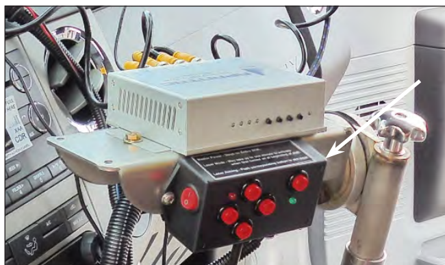
Laser Guidance Control Panel
