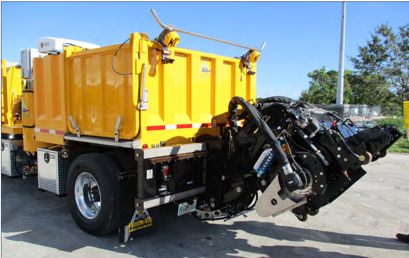
Debris Tank & Door
