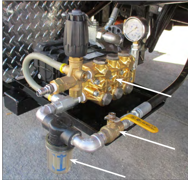
High Pressure Pump, Strainer & Supply Valve
