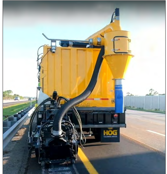
Vacuum Hoses, Cone Shaped Separator with Auger & Access Door
