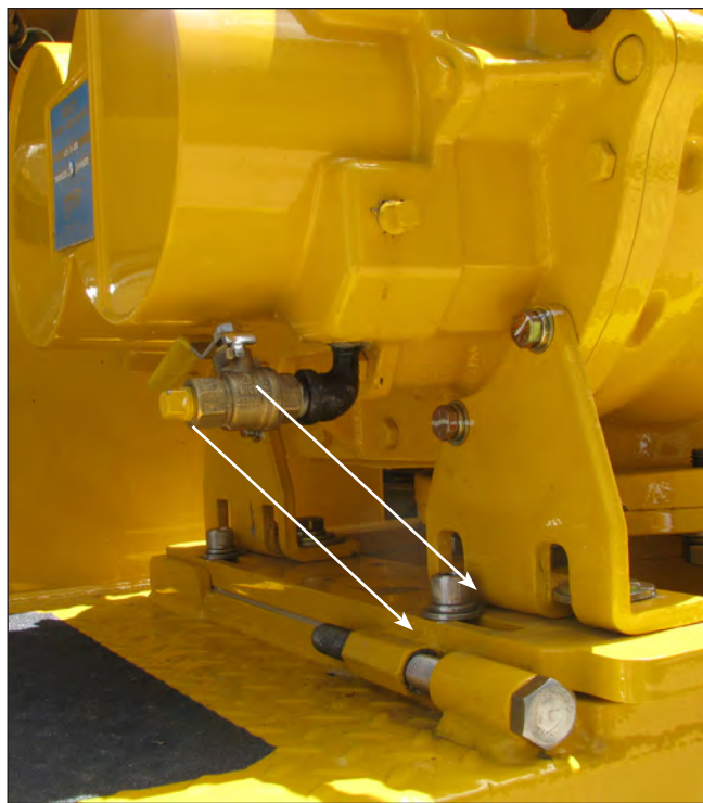
Typical Vacuum Blower Drain Valve & Safety Drain Plug
