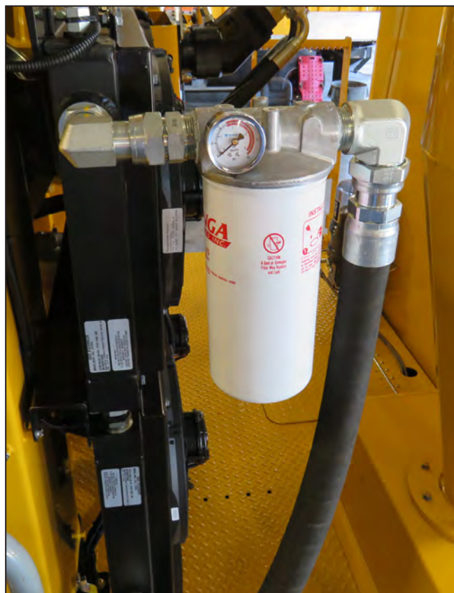
Hydraulic System Low Pressure Filters & Pressure Gauge
