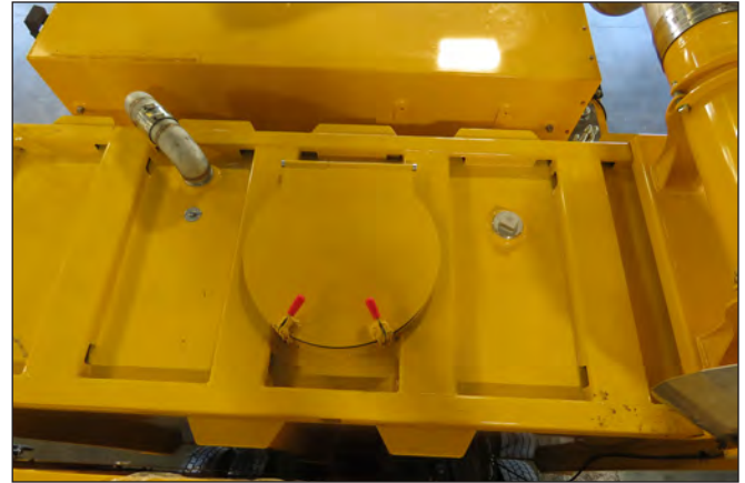
Water Tank Man-Way Hatch
