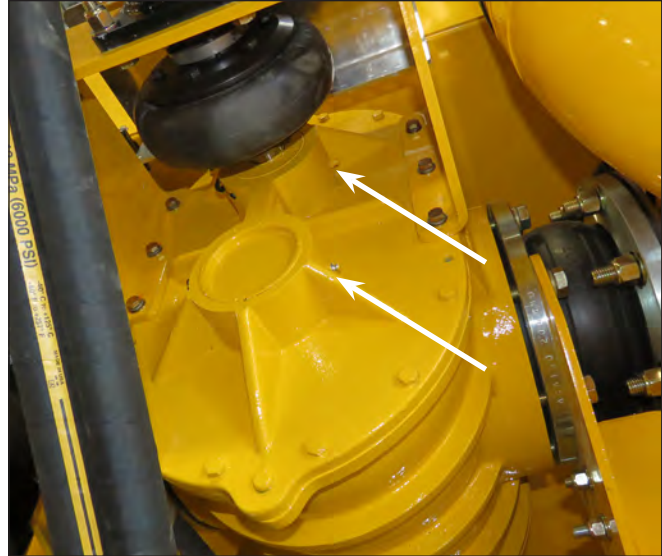
Blower Drive End & Grease Fitting Locations
