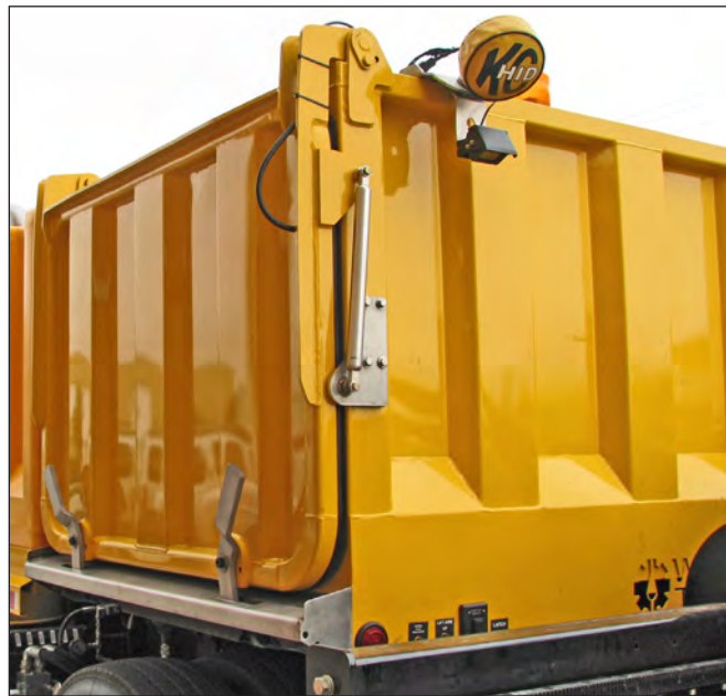
Debris Tank & Debris Tank Door
