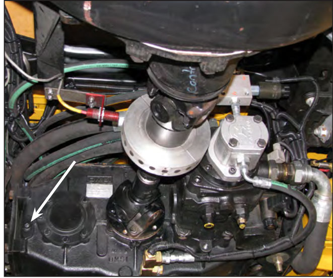
OMSI Drive Gearbox-Fluid Level Plug Location
