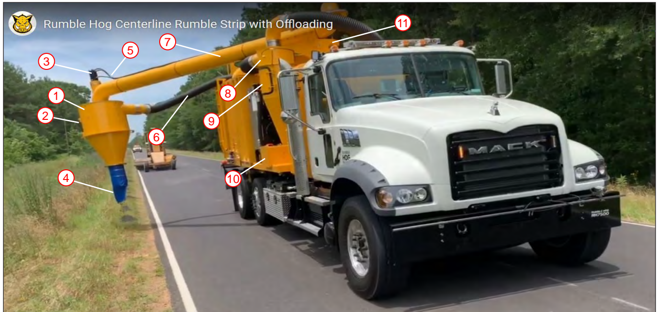
Optional Debris Recovery System With Continuous Off-Loading System
