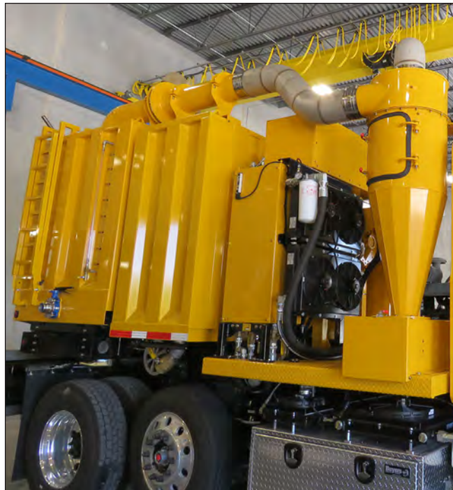
Vacuum Tube - Debris Tank to Cyclonic Separator
