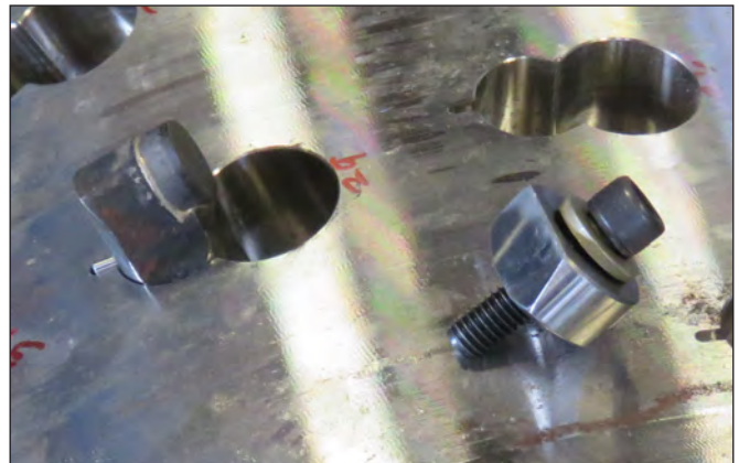
Bolt Washer & Wedge Note that the tooth is in position in the socket
