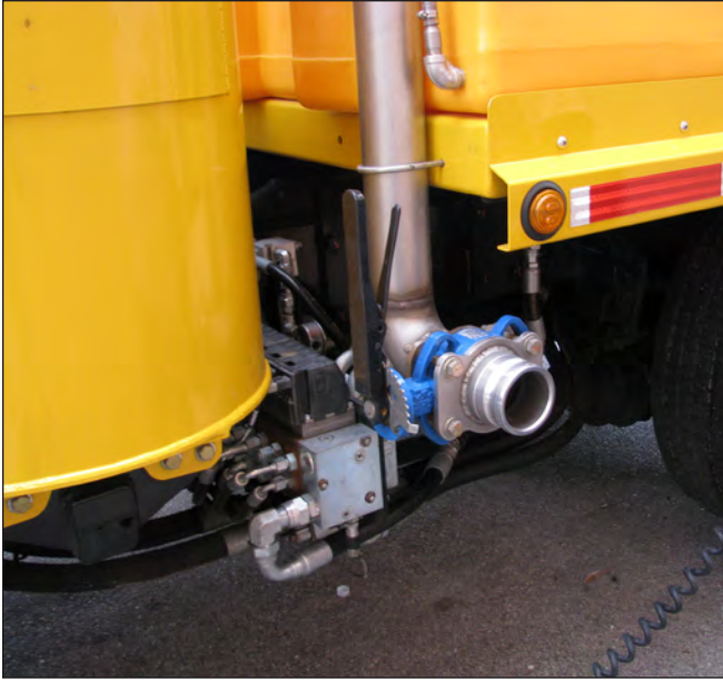
Clean Water Fill Fitting & Valve
