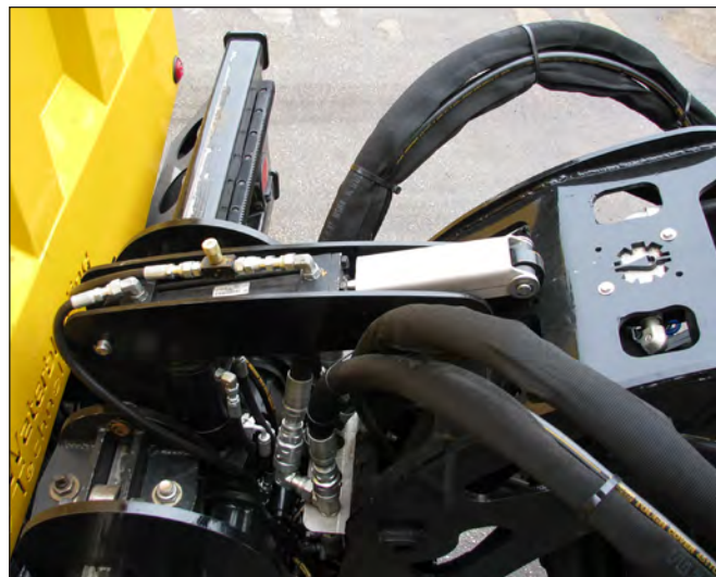
Locking Arm Latched To Lift Arm & Secured With Locking Plate
