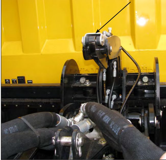
Locking Arm Released From Lift Arm With Latch Closed For Operation
