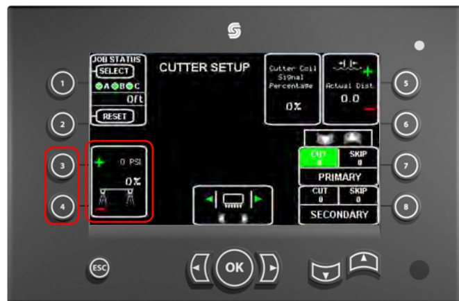
CUTTER SETUP Screen - Setting Spray Nozzle Water Pressure
