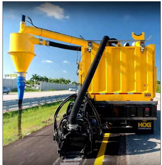
Debris Recovery System With Optional Continuous Off-Loading System
