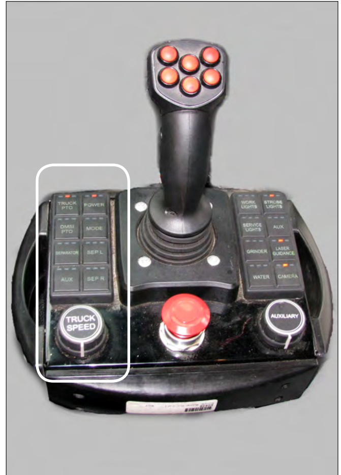
POWER, TRUCK PTO, OMSI PTO & MODE Switches TRUCK SPEED Dial
