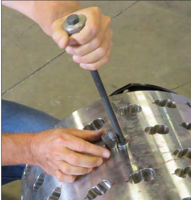
Remove Wedge & Tooth With A Slide Hammer
