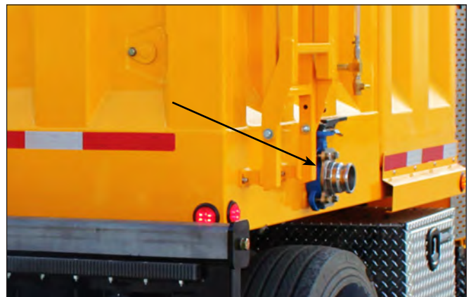
Debris Tank Drain Valve
