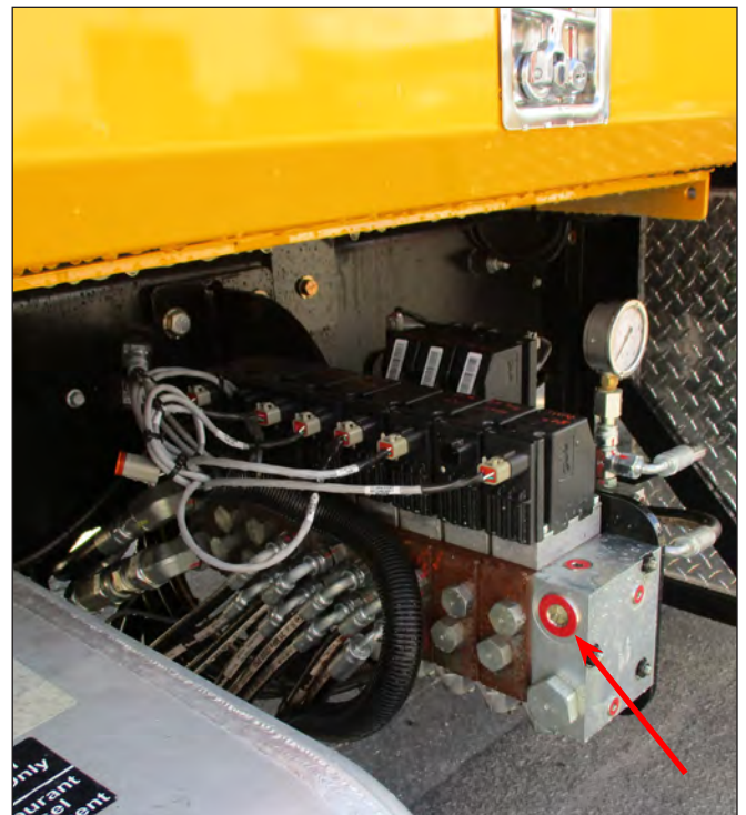
Hydraulic Manifold & Manual Down Pressure Valve
