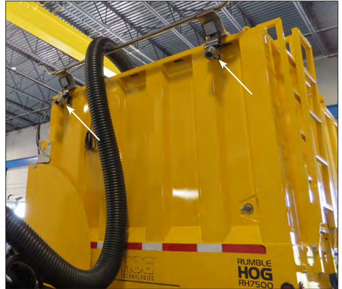
Rear Cameras On Each Side Of Debris Tank
