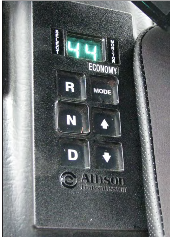
Automatic Transmission Gear Selector & LED Screen OMSI PTO & MODE Switches ON & 4/4 Lockup Displayed
