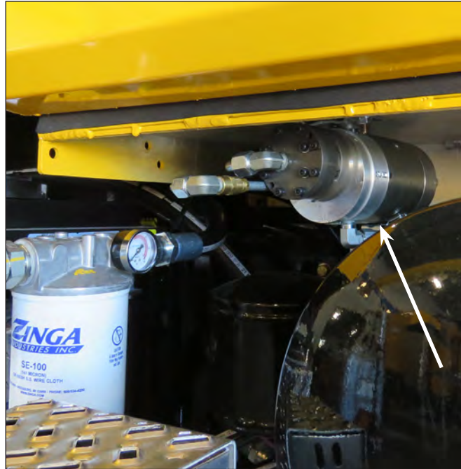
Electric Hydraulic Pump
