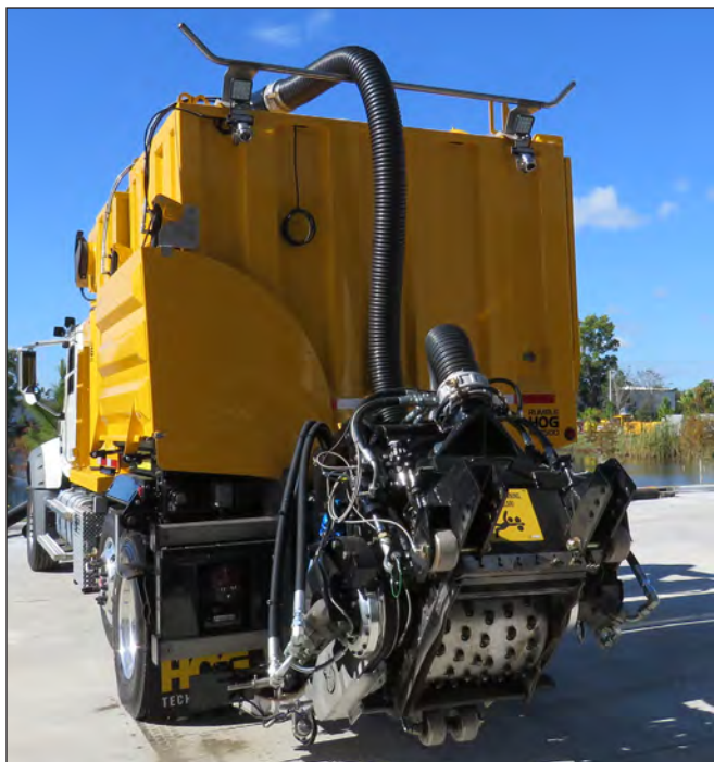
Vacuum Hose - Debris Tank to Cutter
