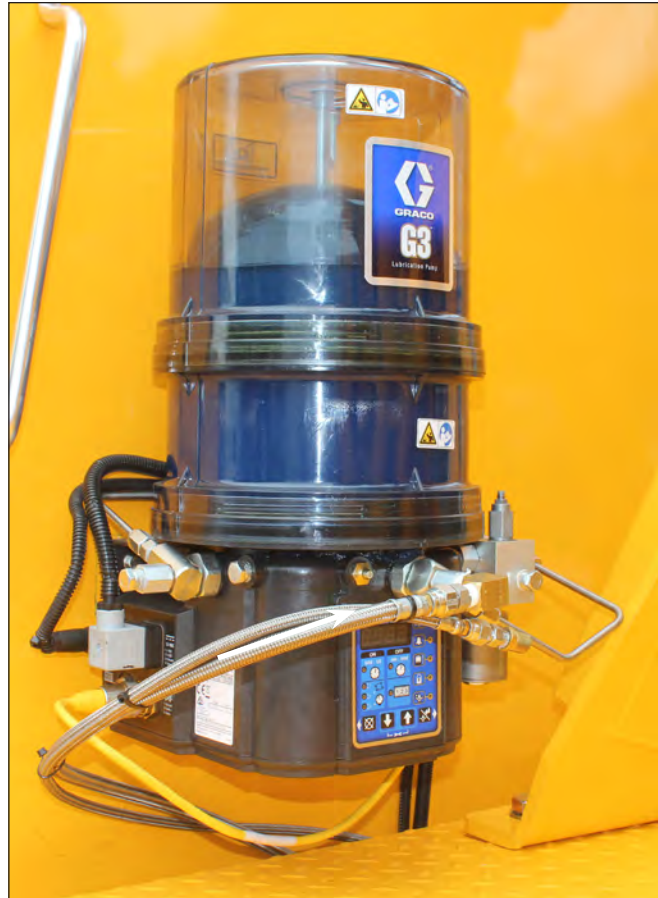
Auto Lube Grease Pump & Reservoir Fill Fitting
