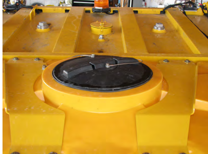
Rear Clean Water Tank Man-Way & Wastewater Bladder
