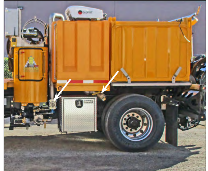
Clean Water Tank Fill & Drain Valves
