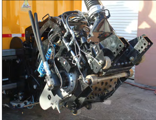
Cutter Configured For Rumble Strips
