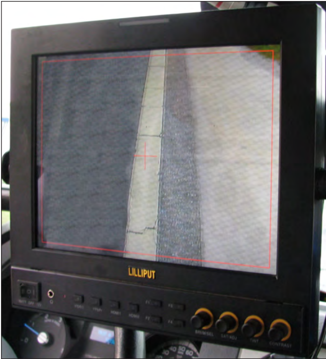
Forward Camera Video Monitor With Alignment Indicator On Reference Line
