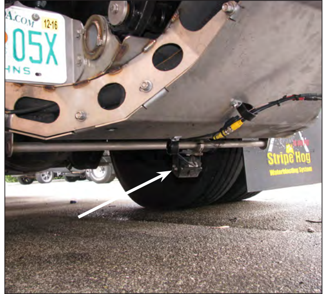
Rear Guidance Camera Forward of Cutting Drum
