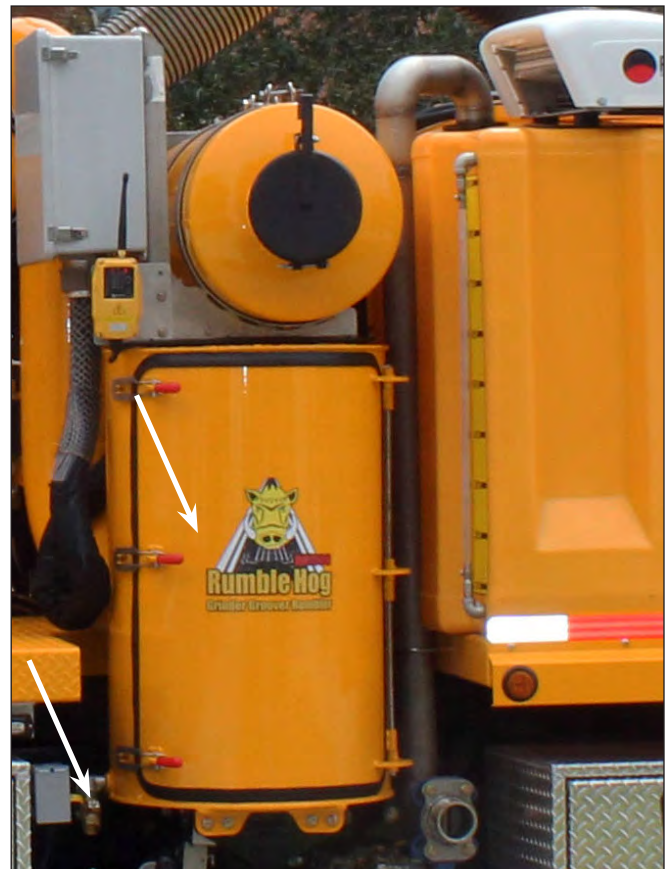
Vacuum Filter Canister, Door & Drain Valve
