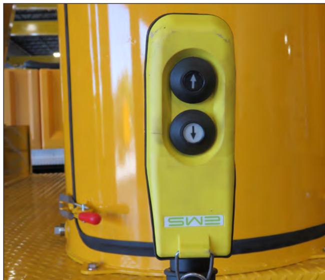
Remote Switch Control
