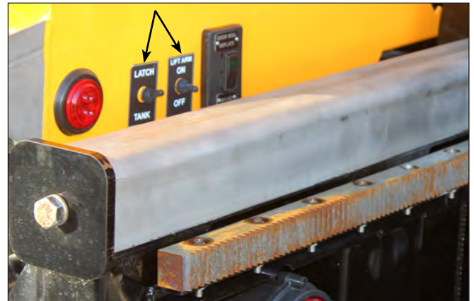
Rear Control Switches
