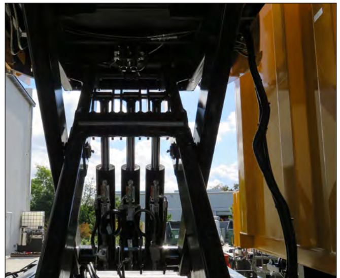
Debris Tank Lift Cylinders
