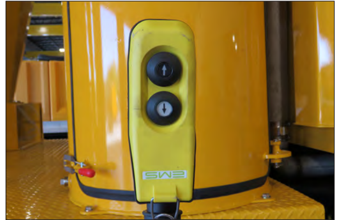
Remote Control Switches
