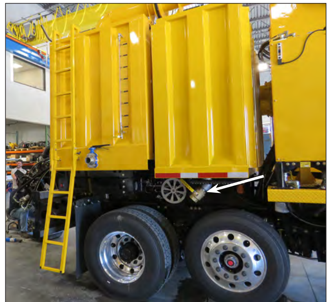
Water Tank Drain Valve
