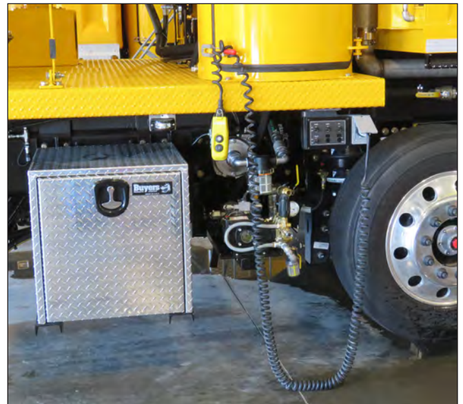
Remote Control Connected to Grey Junction Box
