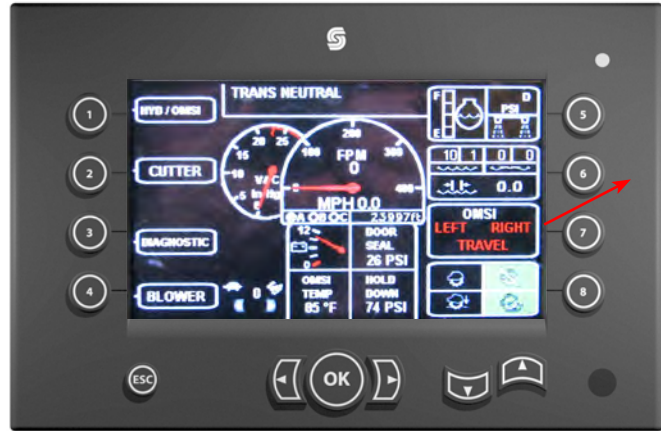
Controller MAIN Screen & Control Buttons Indicating Travel Mode
