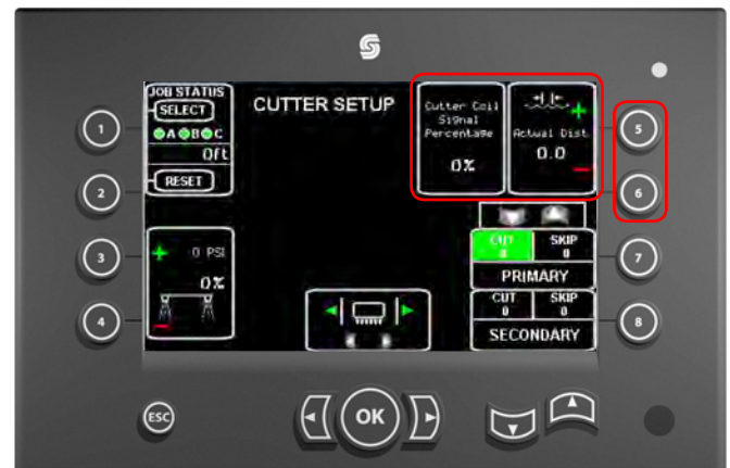
CUTTER SETUP Screen - Setting Cut Spacing
