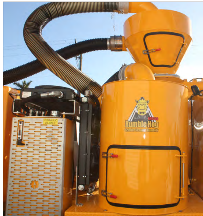
Cone Shaped Primary Separator & Secondary Separator
