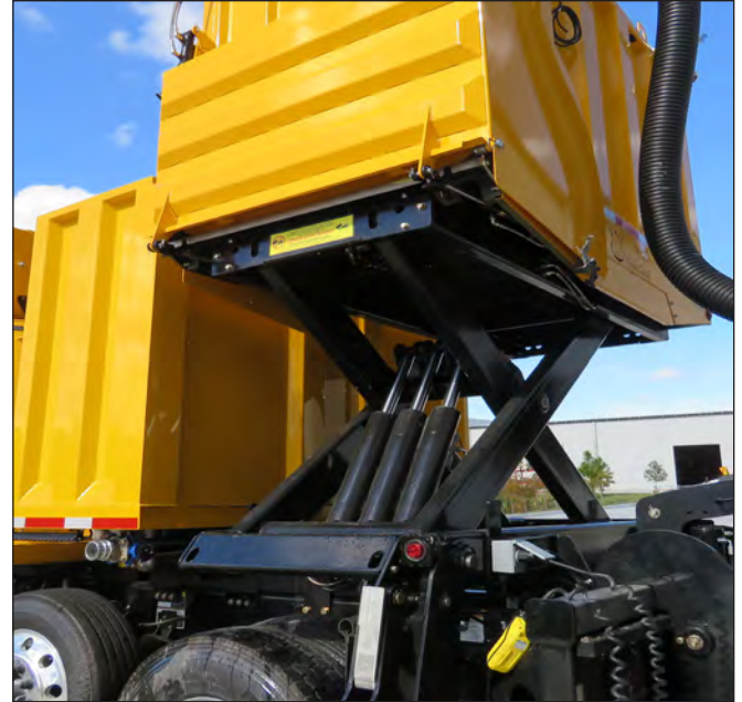
Debris Tank Lift Cylinders & Scissor Linkage
