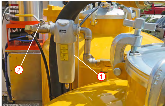
Air Filter/Drier & Pressure Supply Valve
