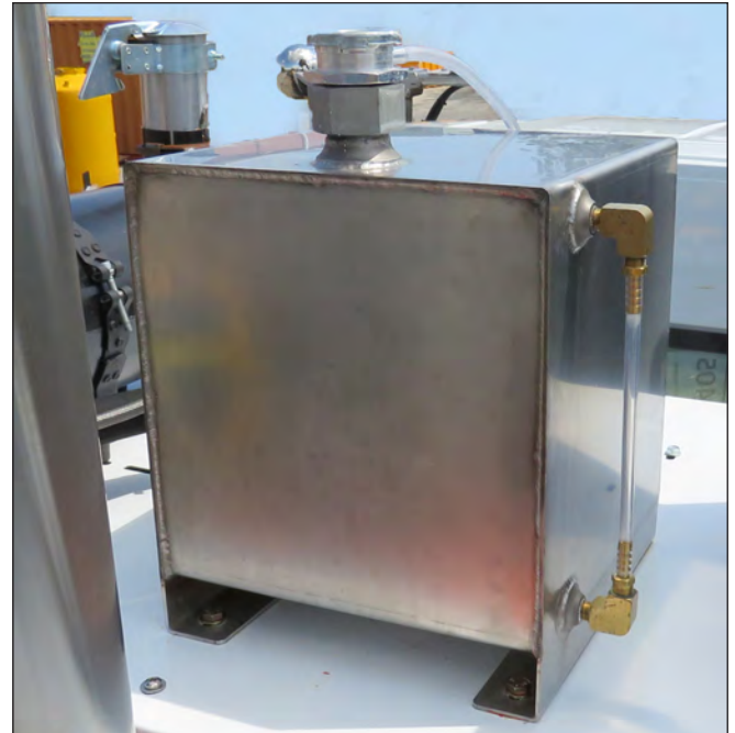
Antifreeze Expansion tank, Pressure Cap & Sight Gauge
