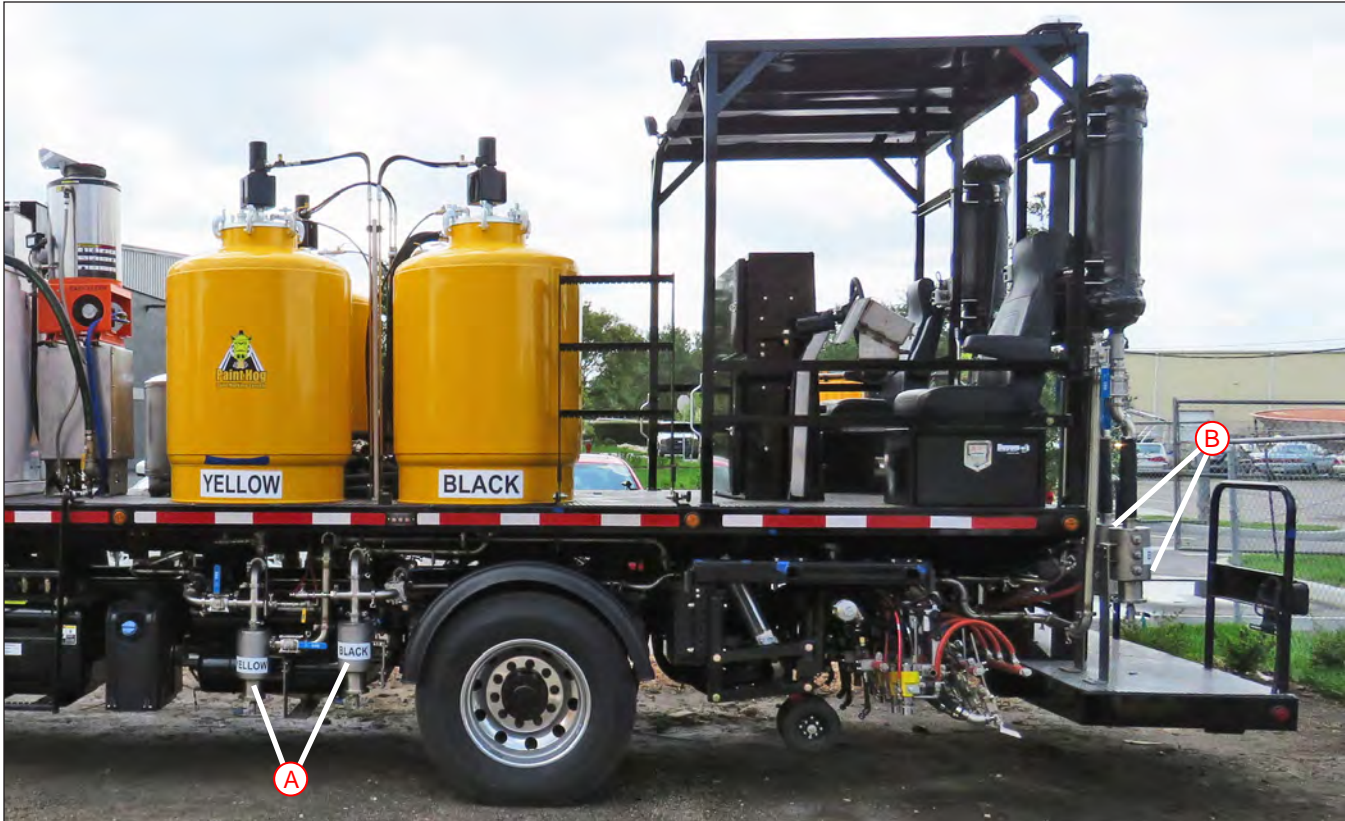
Driver Side Primary & Secondary Filters A. Primary Filters / B. Secondary Filters
