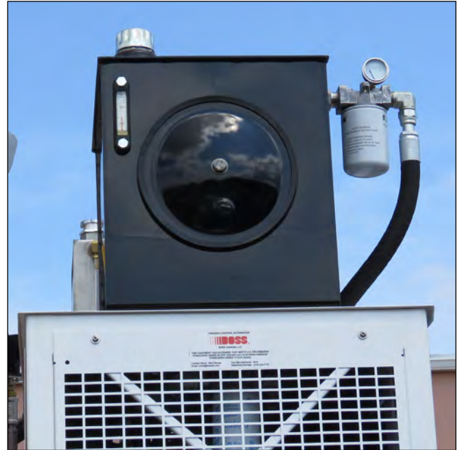
Hydraulic Reservoir, Sight Gauge & Filter
