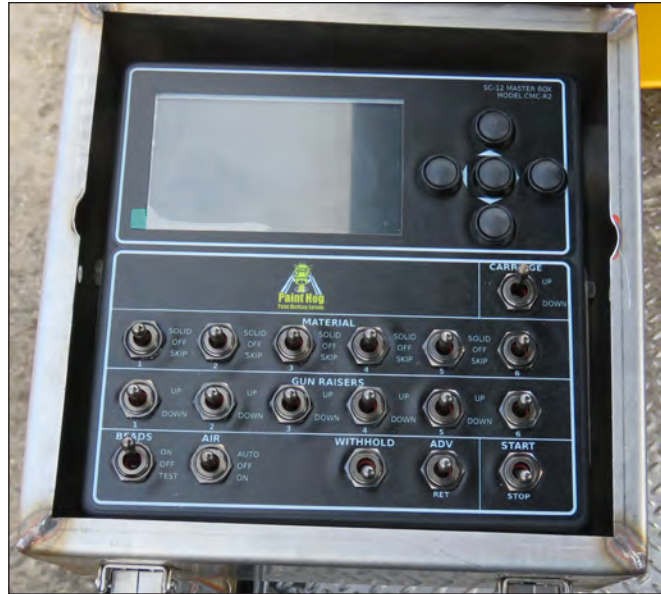
Spray Gun Control Panel Switches & Skip Line Controller
