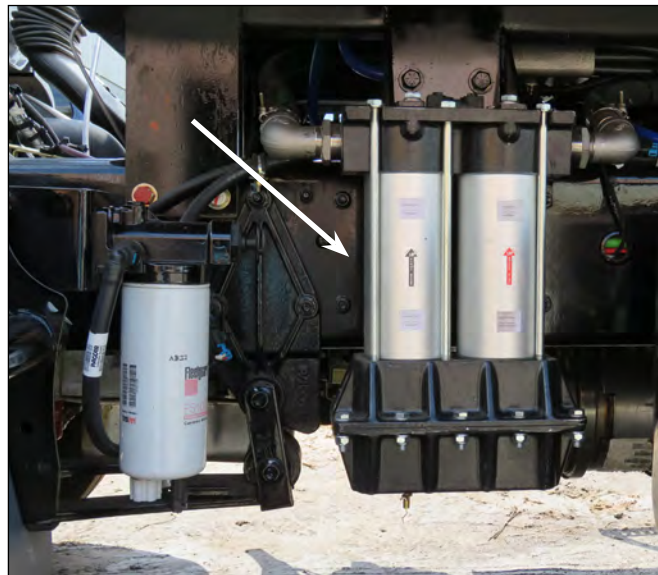
Primary Moisture Separating Air Filters
