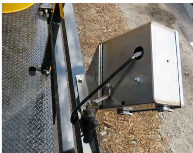
Spray Gun Controller Swung Up To Provide Walk Around Clearance
