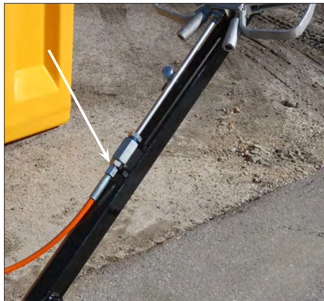
UHP Control Valve To Thru-Shaft Pump Hose Connection & Fittings
