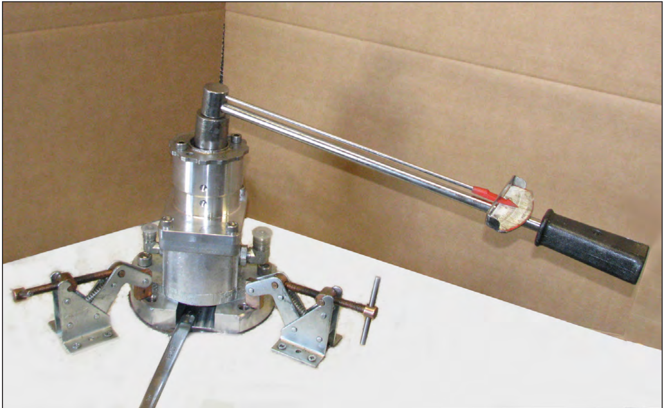
Figure 12: Thrust housing cap bolts securing the spanner tool are snug and a torque wrench and 1 1/8" deep well socket is used to tighten the jam nut to 50 ft lbs.
