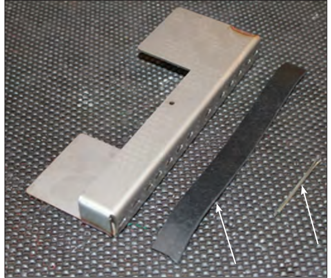
Spray Bar Protector, Cotter Pin & Gasket
