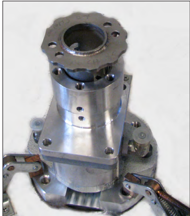
Figure 10: Use spanner to turn spanner nut.
