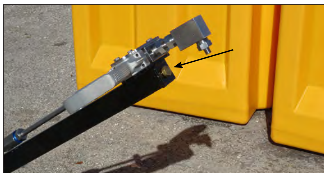
Hydraulic Brake Fluid Level/Fill Plug
