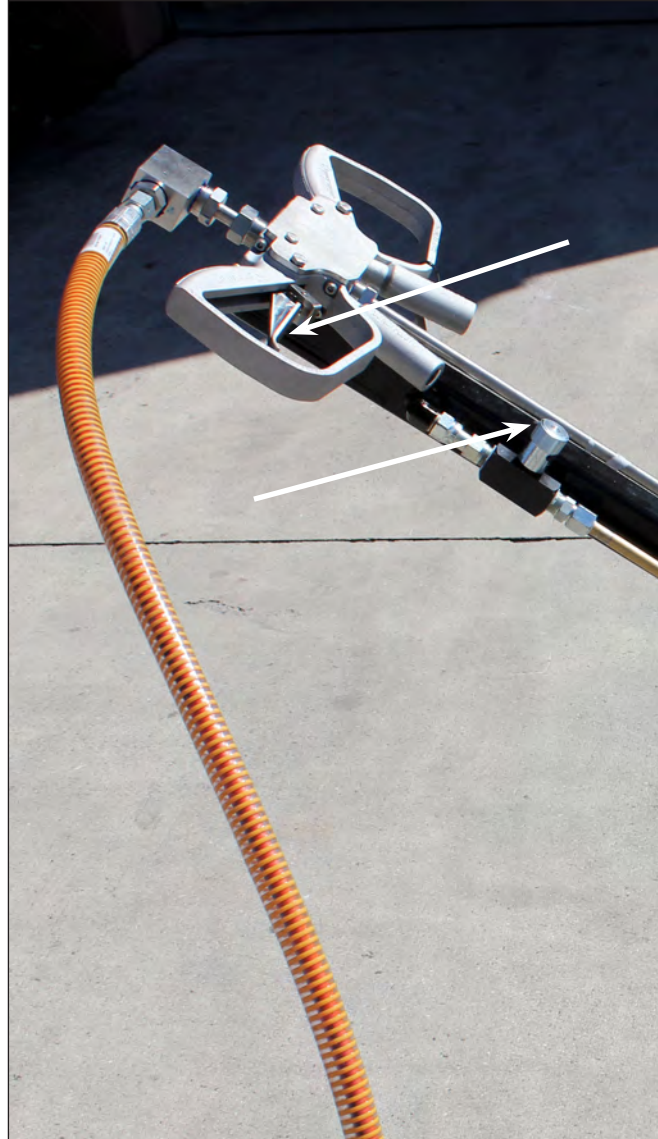
Ground Hog UHP/Dump Valve Control Lever & Spray Bar Rotation Speed Control Needle Valve
