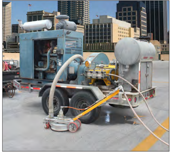
Typical Power System Make sure it is shutdown & perform Lockout/Tagout procedures before servicing equipment.
