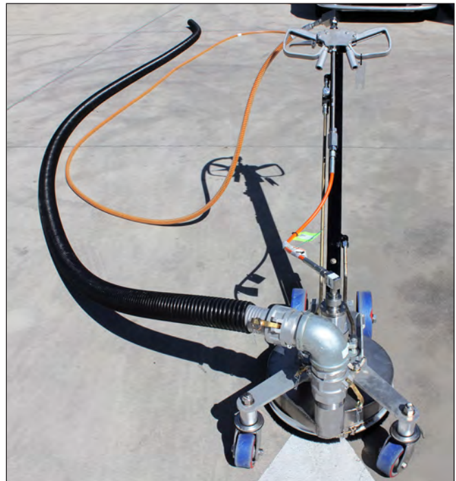
Ground Hog With Vacuum & UHP Hoses Connected Remove UHP & vacuum hoses from Ground Hog before performing any service.
