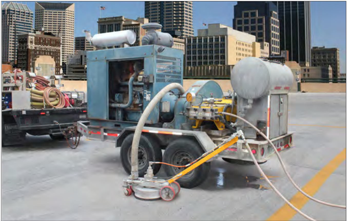
Ground Hog Connected To A Typical UHP & Vacuum Power System - Ready For Operation
