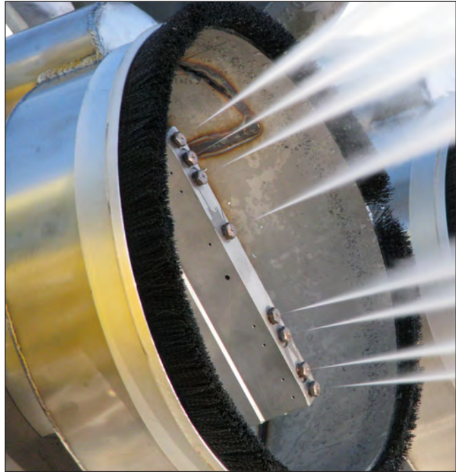
Nozzle Pressure Test - All Nozzles Good
