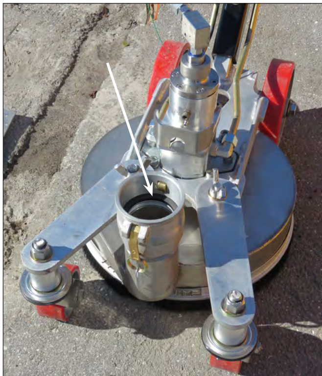
Ground Hog Vacuum Hose Connection & Seal
