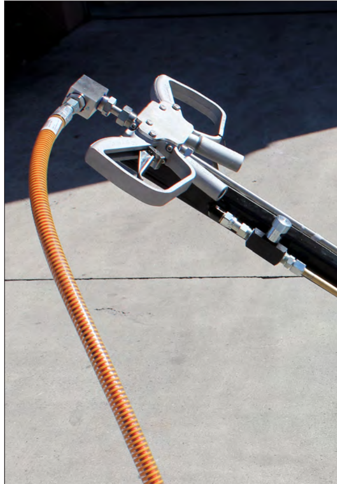
UHP Pump To Ground Hog Hose Connection & Fittings
