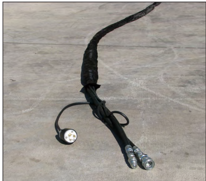
Hydraulic Hoses and Electrical Control Harness w/ anti-chaffing Typical Power System End w/ Quick Connectors
