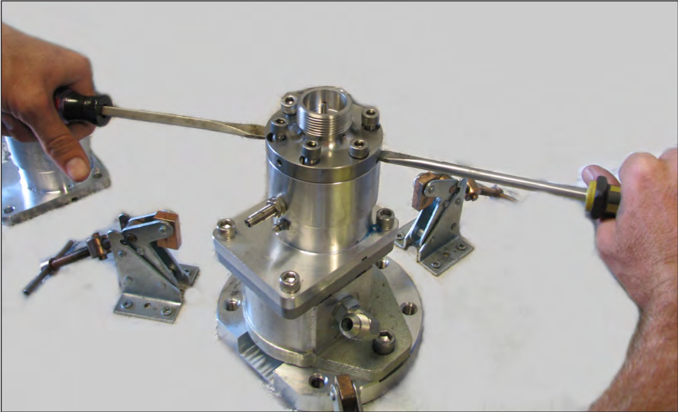
Figure 5: Use two medium flat head screwdrivers to remove the thrust housing cap. Note that the bolts are loose and left in place to prevent thrust housing cap from falling and being damaged during removal.
