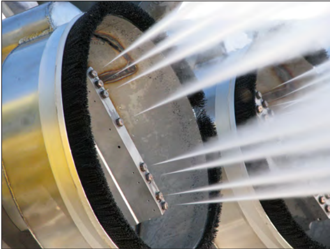
Typical Good Nozzles with a Tight Cohesive Stream Shown on Hog Head Spray Bar
