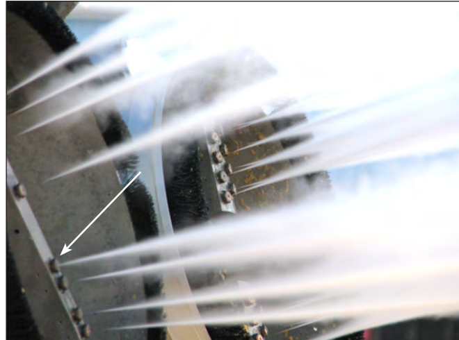
Typical Bad Nozzle - Note Stream Fans Out at Nozzle Shown on Hog Head Spray Bar
