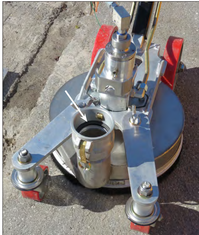
Vacuum Hose Connection Notice seal inside connection. Always make sure the seal is in place before connecting the vacuum hose.
