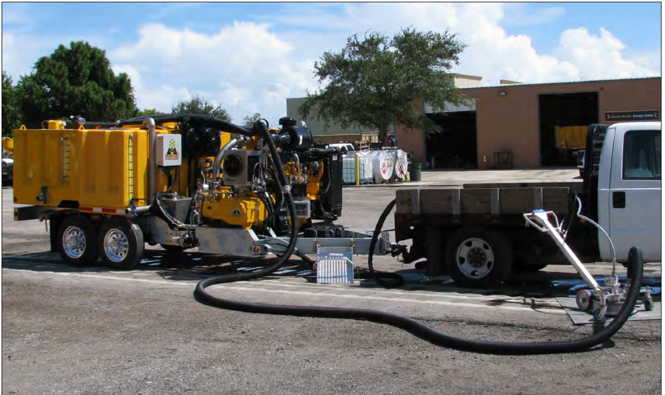
Ground Hog Connected To A Trailer Mounted Waterblasting UHP & Vacuum Power System - Ready For Operation
