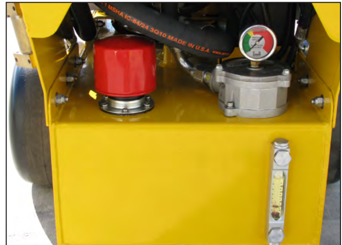
Hydraulic Oil Filter Pressure Gauge, Filter Canister & Fill Cap
