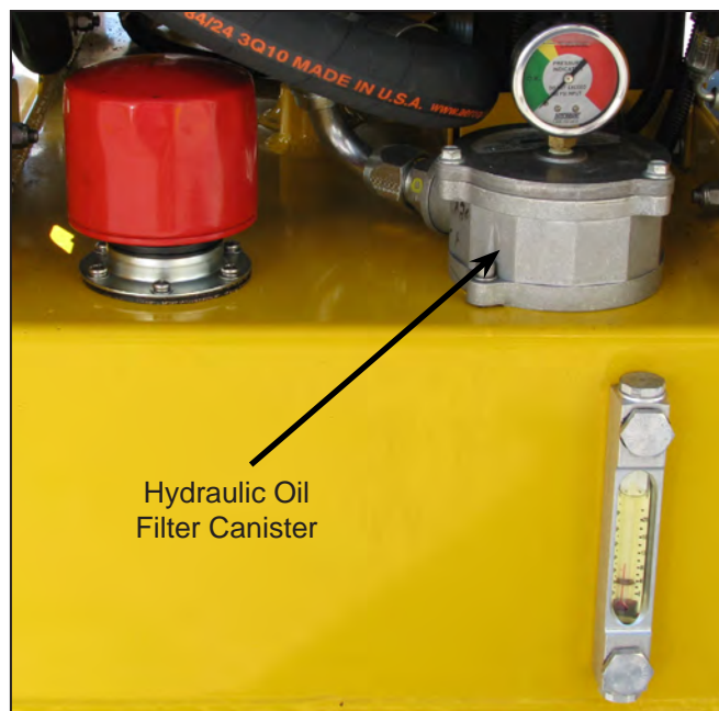
Hydraulic Oil Filter Pressure Gauge, Oil Fill Cap Oil Level Sight Glass & Thermometer
